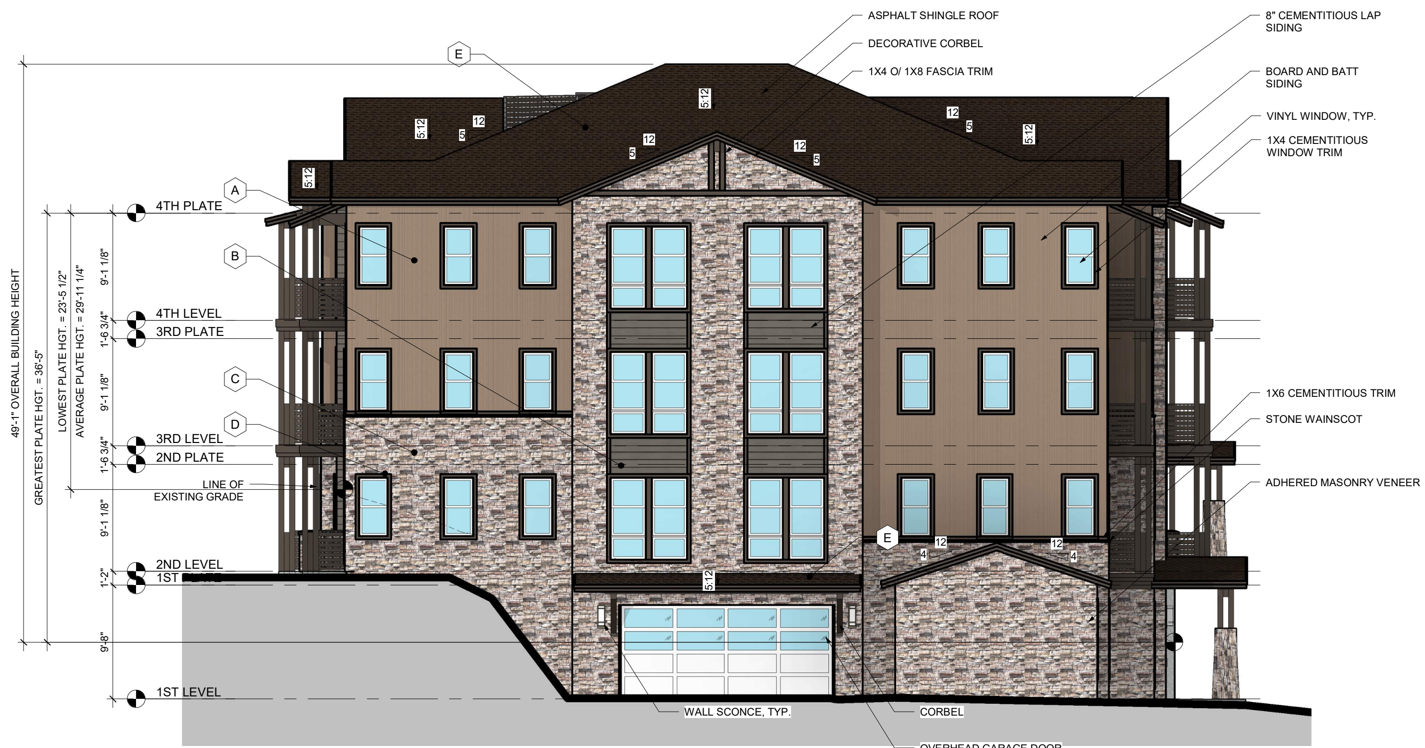
1 BUILDING 1 (TYPE 1A) - FRONT ELEVATION 1/8" = 1'-0"
