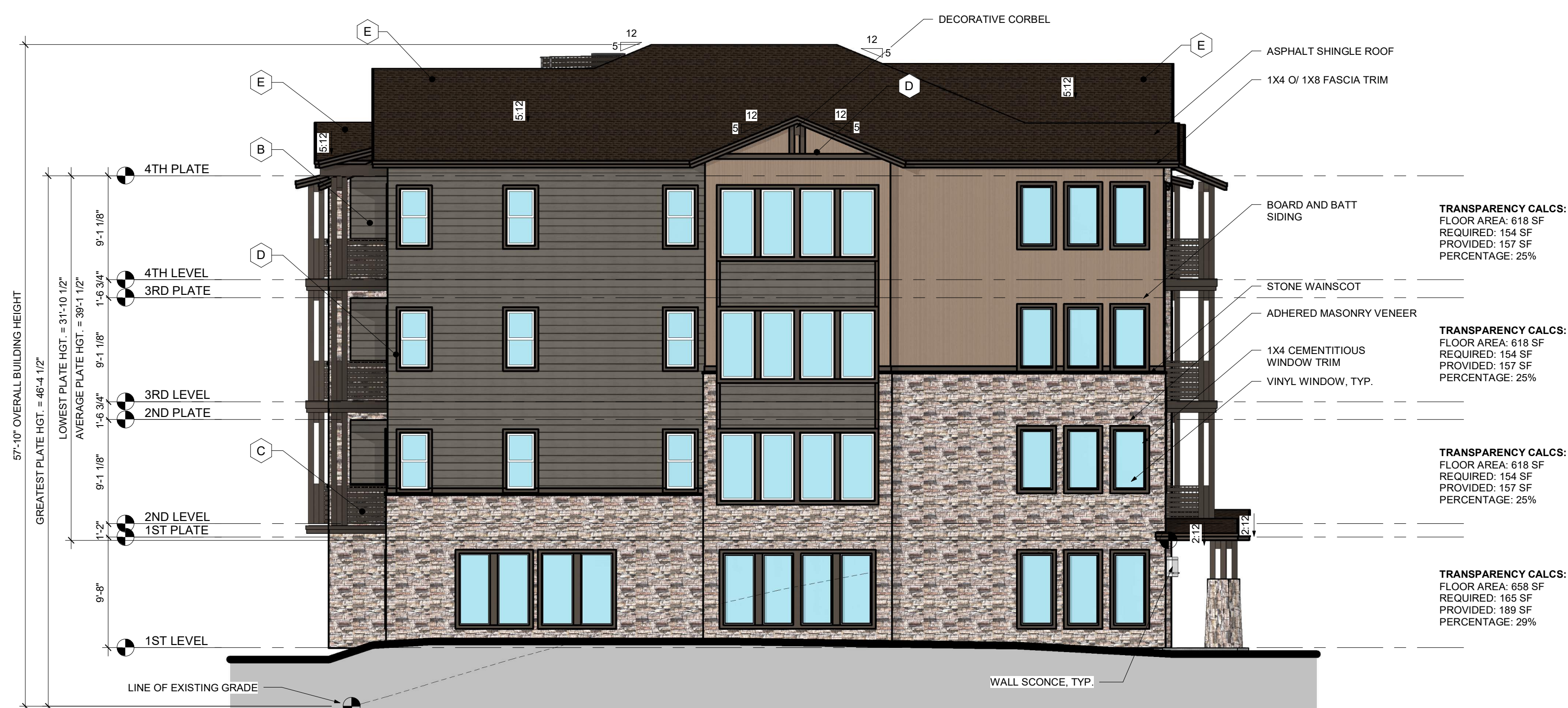
1 BUILDING 7 (TYPE 2) - FRONT ELEVATION 1/8" = 1'-0"
