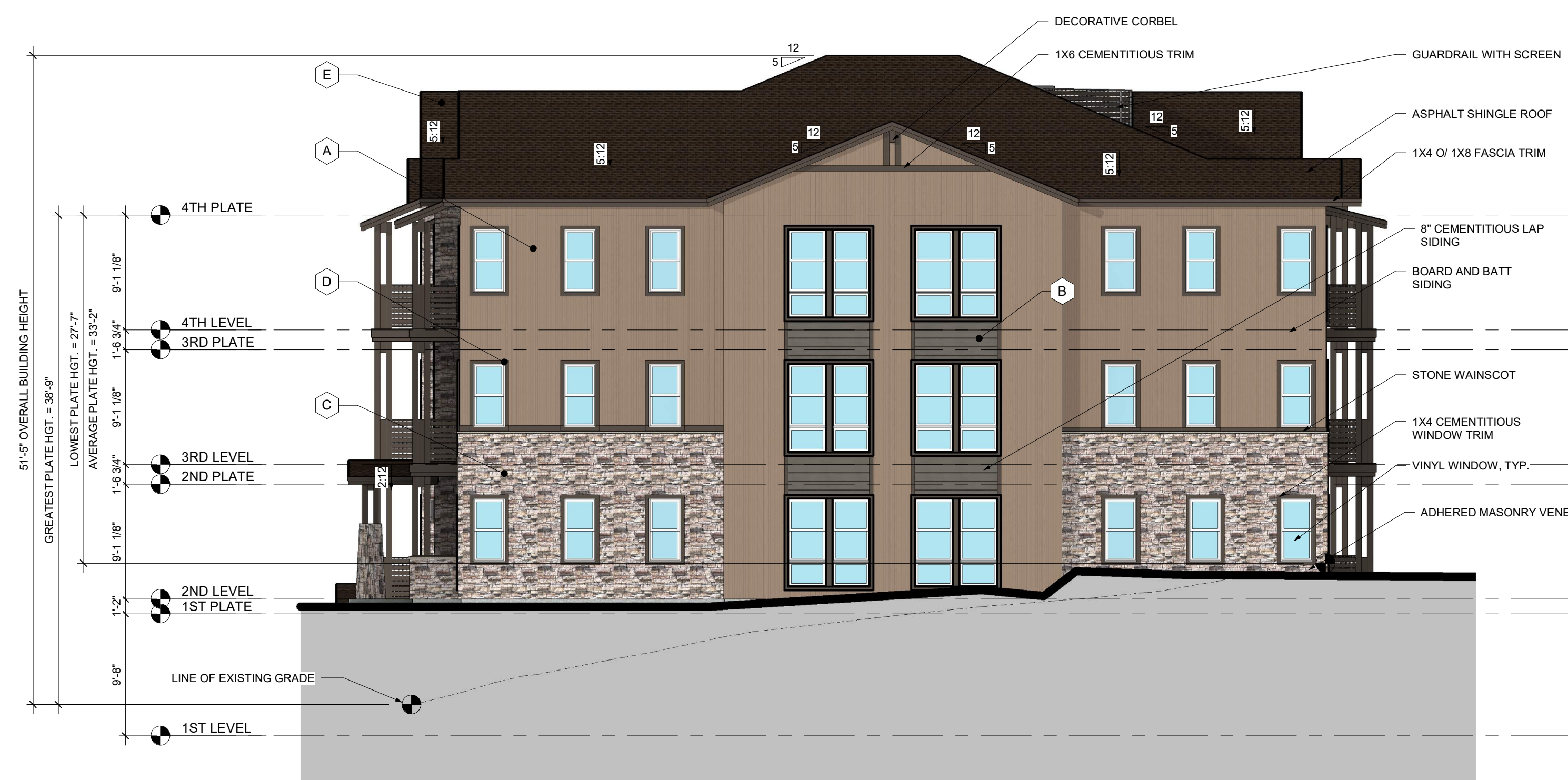
1 BUILDING 1 (TYPE 1A) - REAR ELEVATION 1/8" = 1'-0"
