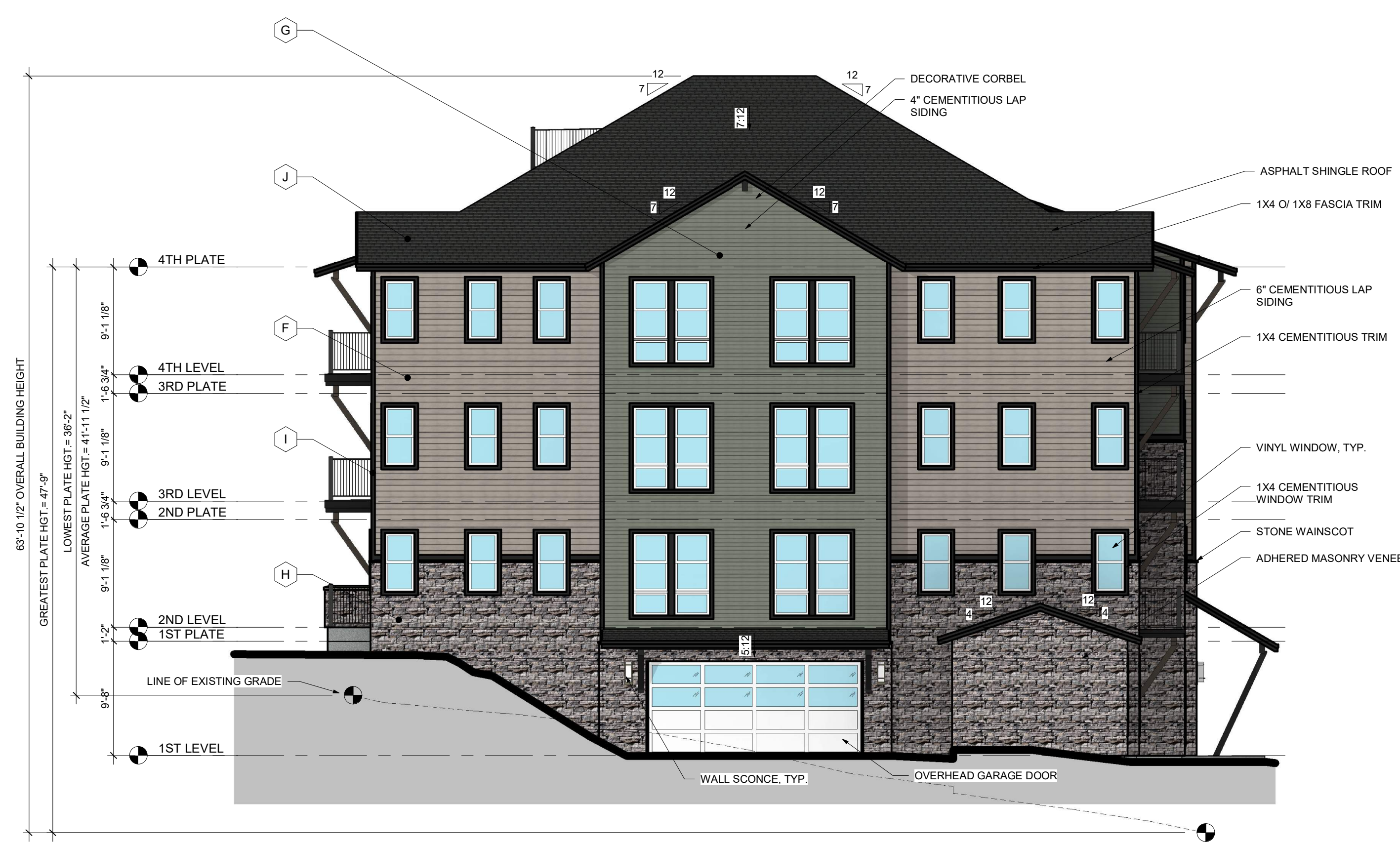
1 BUILDING 2 (TYPE 1B) - FRONT ELEVATION 1/8" = 1'-0"
