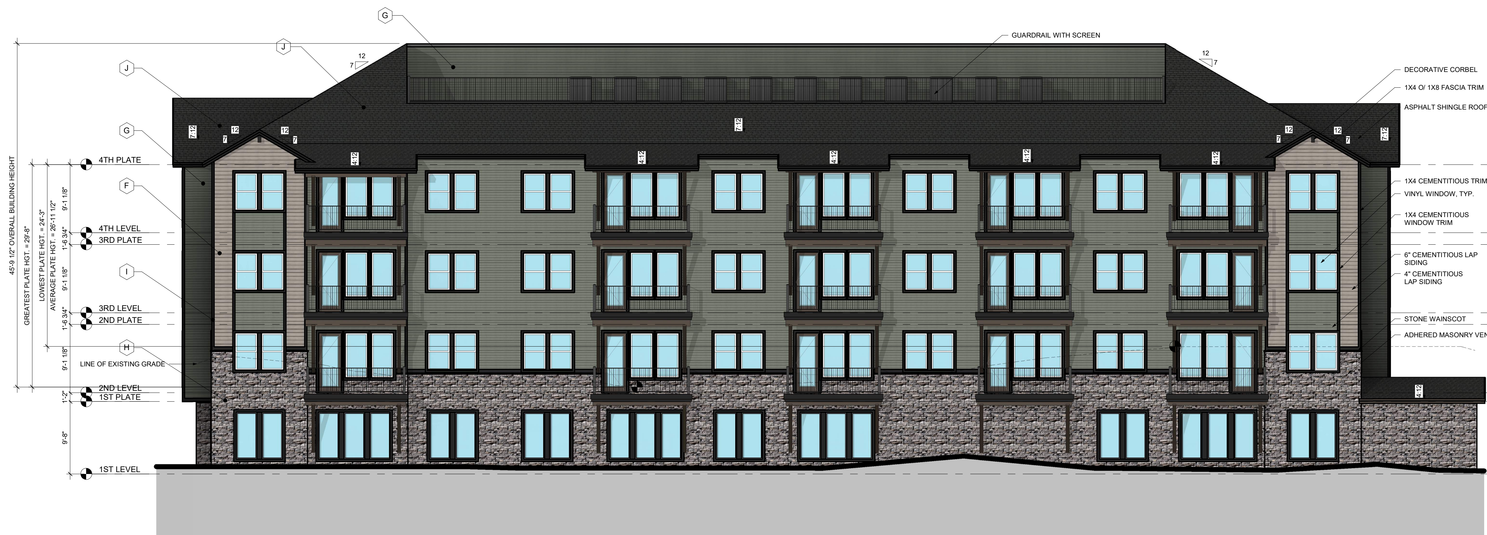
1 BUILDING 6 (TYPE 1B) - REAR ELEVATION 1/8" = 1'-0"
