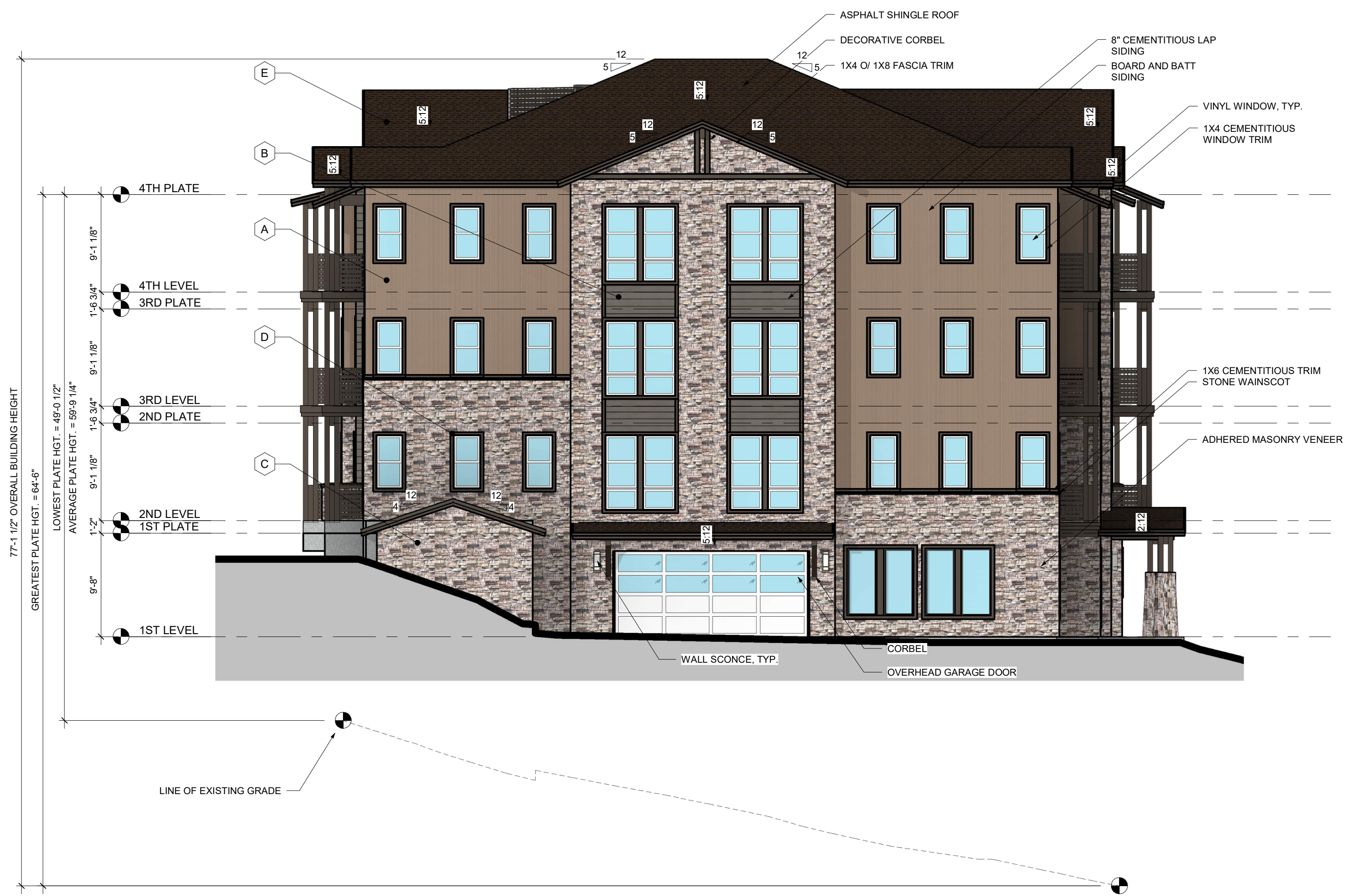
2 BUILDING 5 (TYPE 1A) - LEFT ELEVATION 1/8" = 1'-0"
