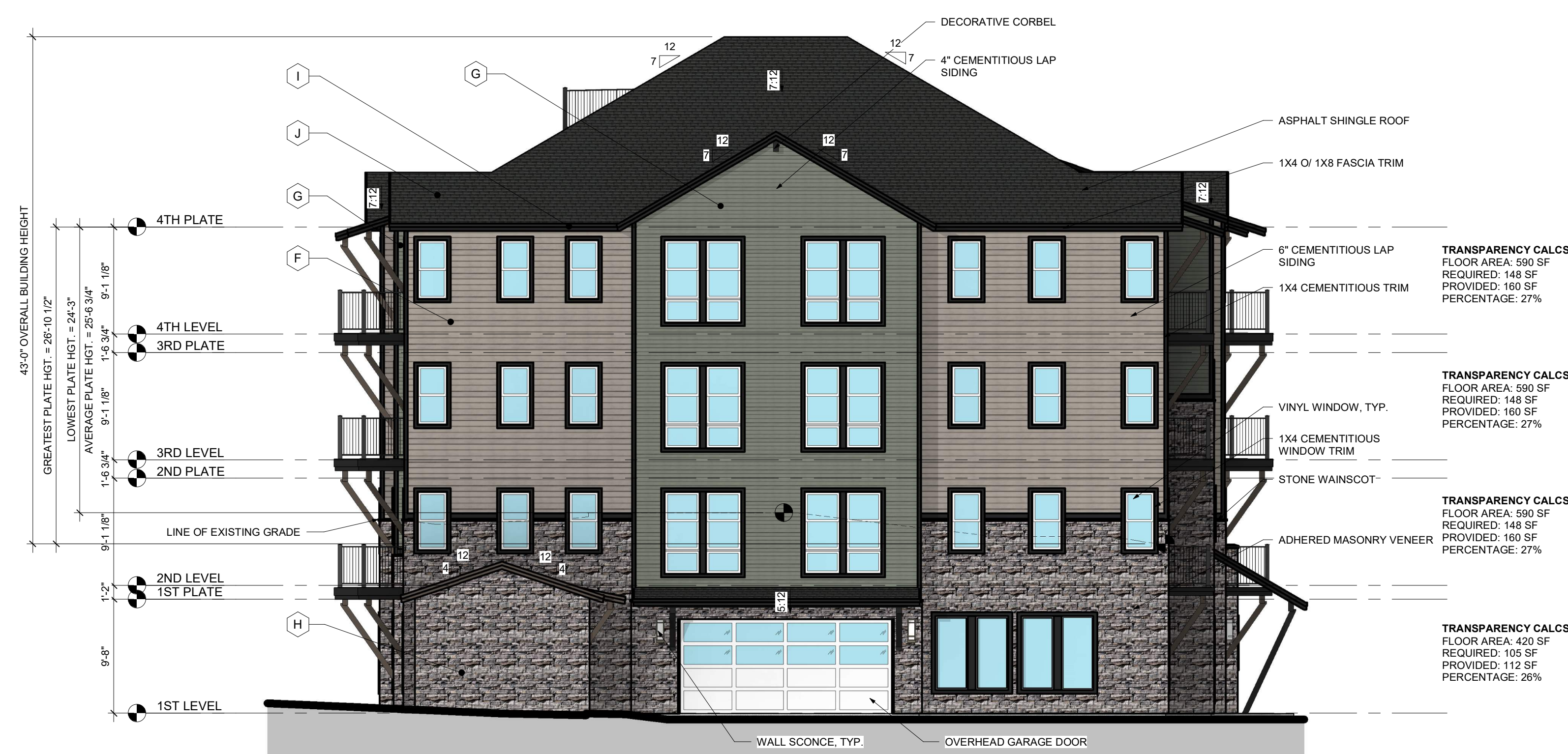
1 BUILDING 6 (TYPE 1B) - FRONT ELEVATION 1/8" = 1'-0"
