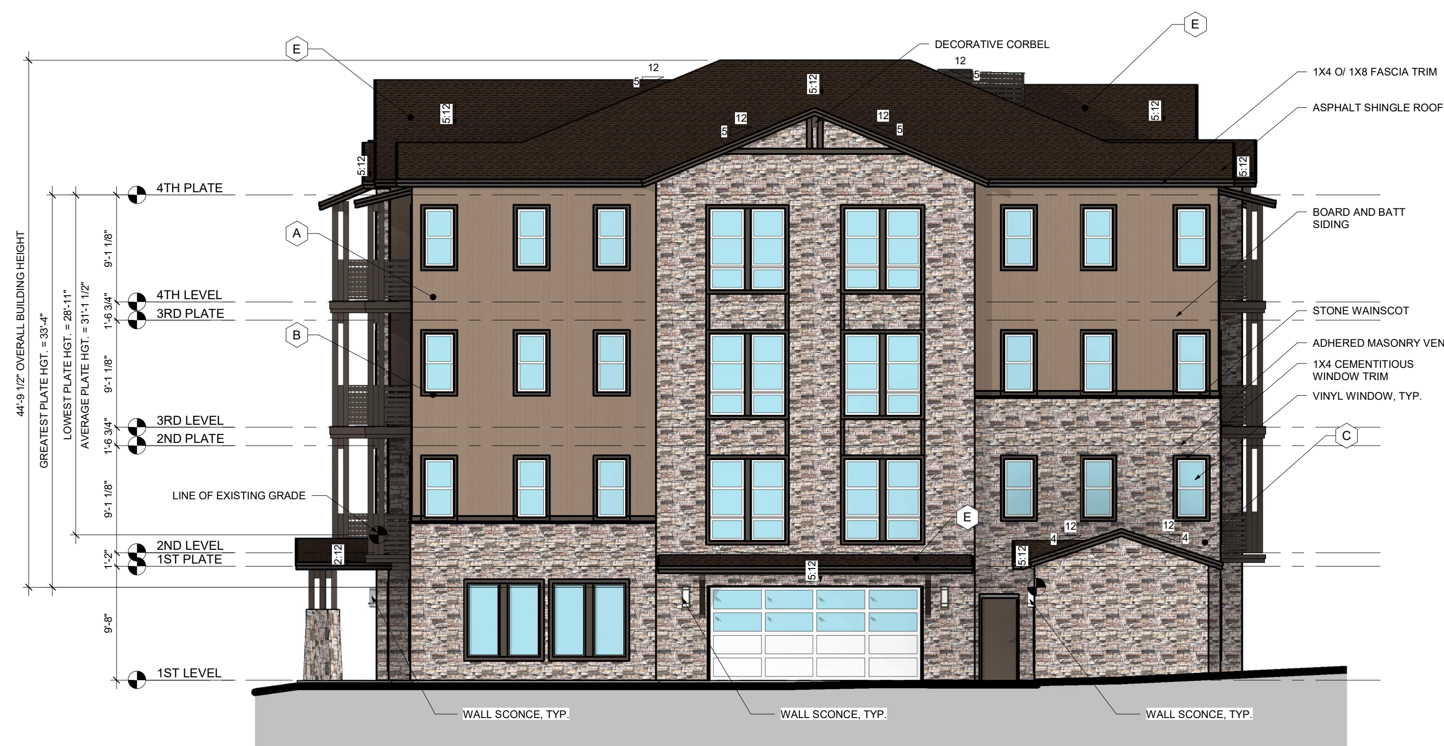
1 BUILDING 7 (TYPE 2) - REAR ELEVATION 1/8" = 1'-0"
