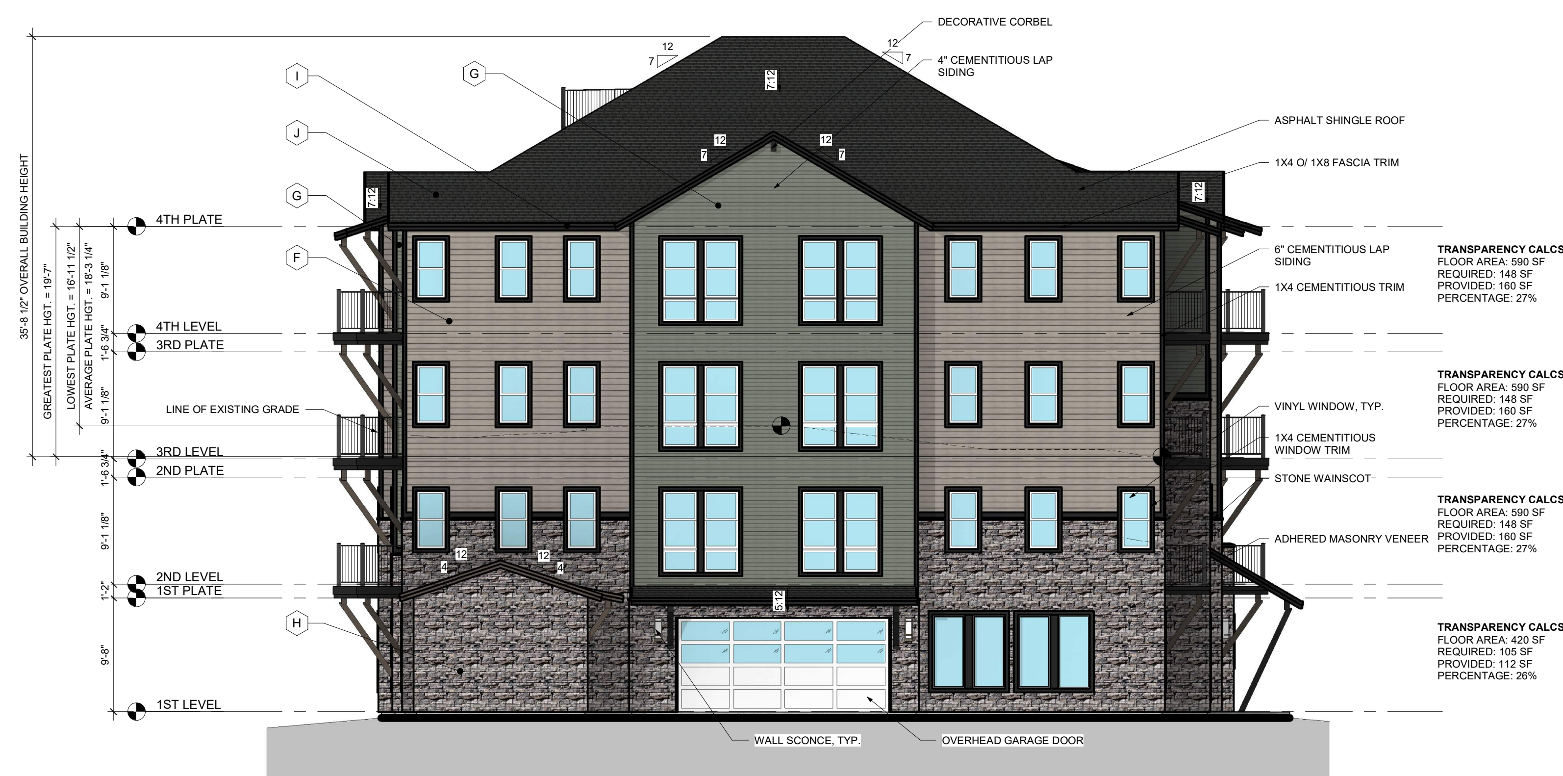
1 BUILDING 6 (TYPE 1B) - FRONT ELEVATION 1/8" = 1'-0"
