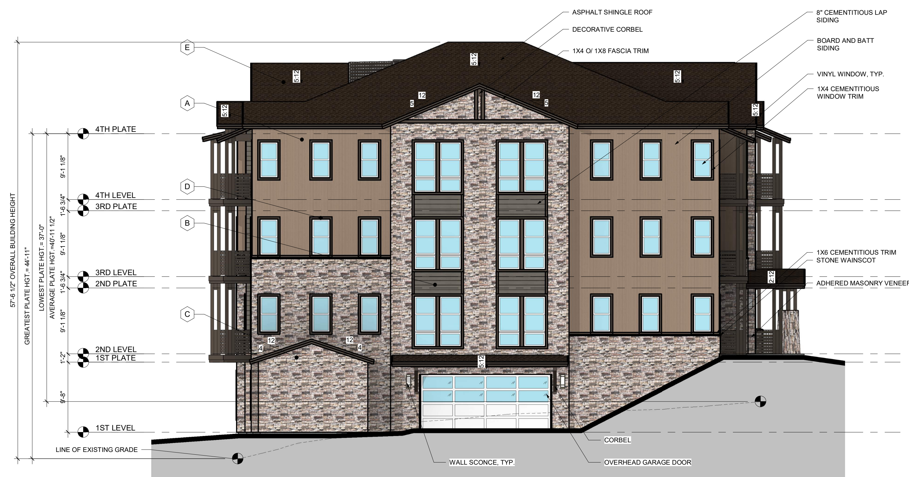
1 BUILDING 3 (TYPE 1A) - FRONT ELEVATION 1/8" = 1'-0"
