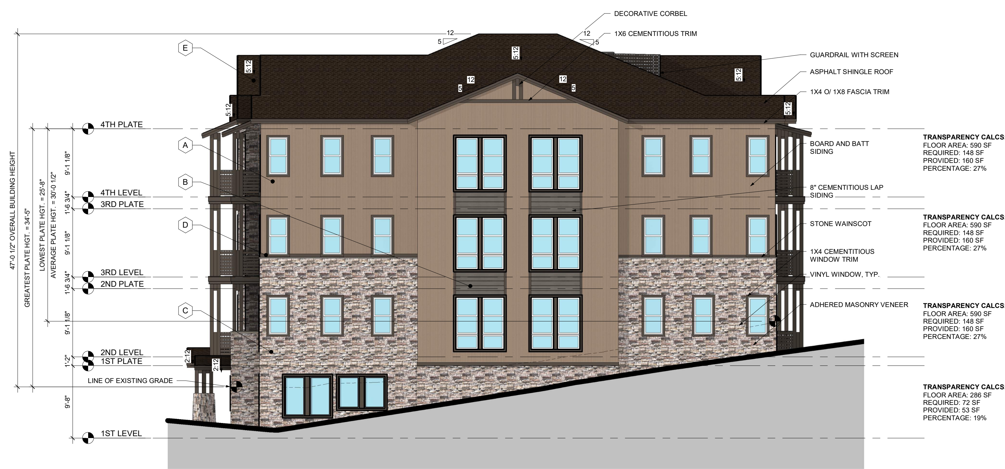
1 BUILDING 5 (TYPE 1A) - REAR ELEVATION 1/8" = 1'-0"
