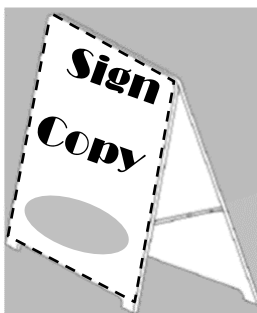
Figure 506-10. Faces that are not parallel, angle \leq 45 degrees
