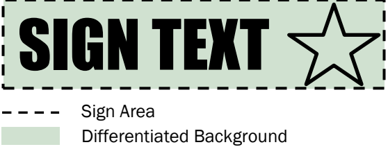
Figure 506-1. Sign Area, Differentiated Background
