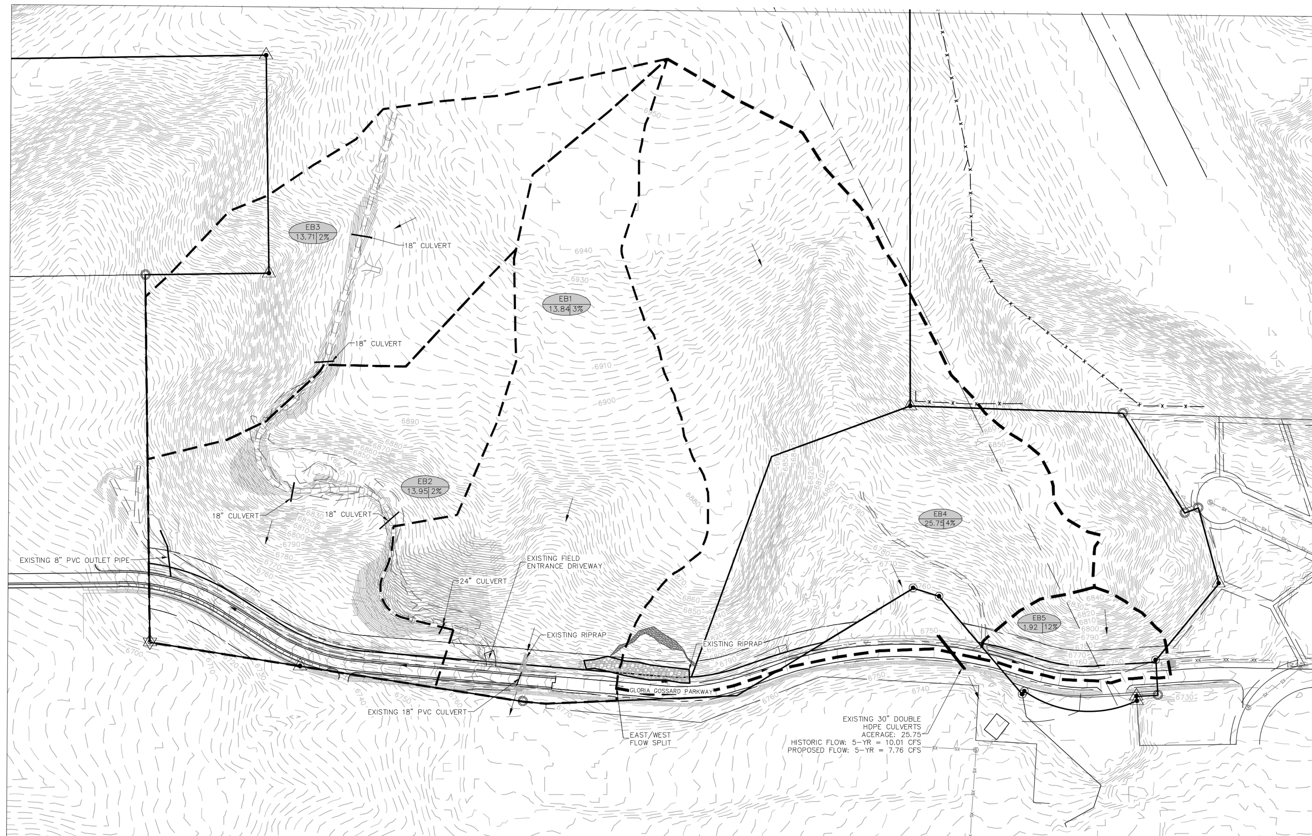
EXISTING DRAINAGE CONDITIONS
