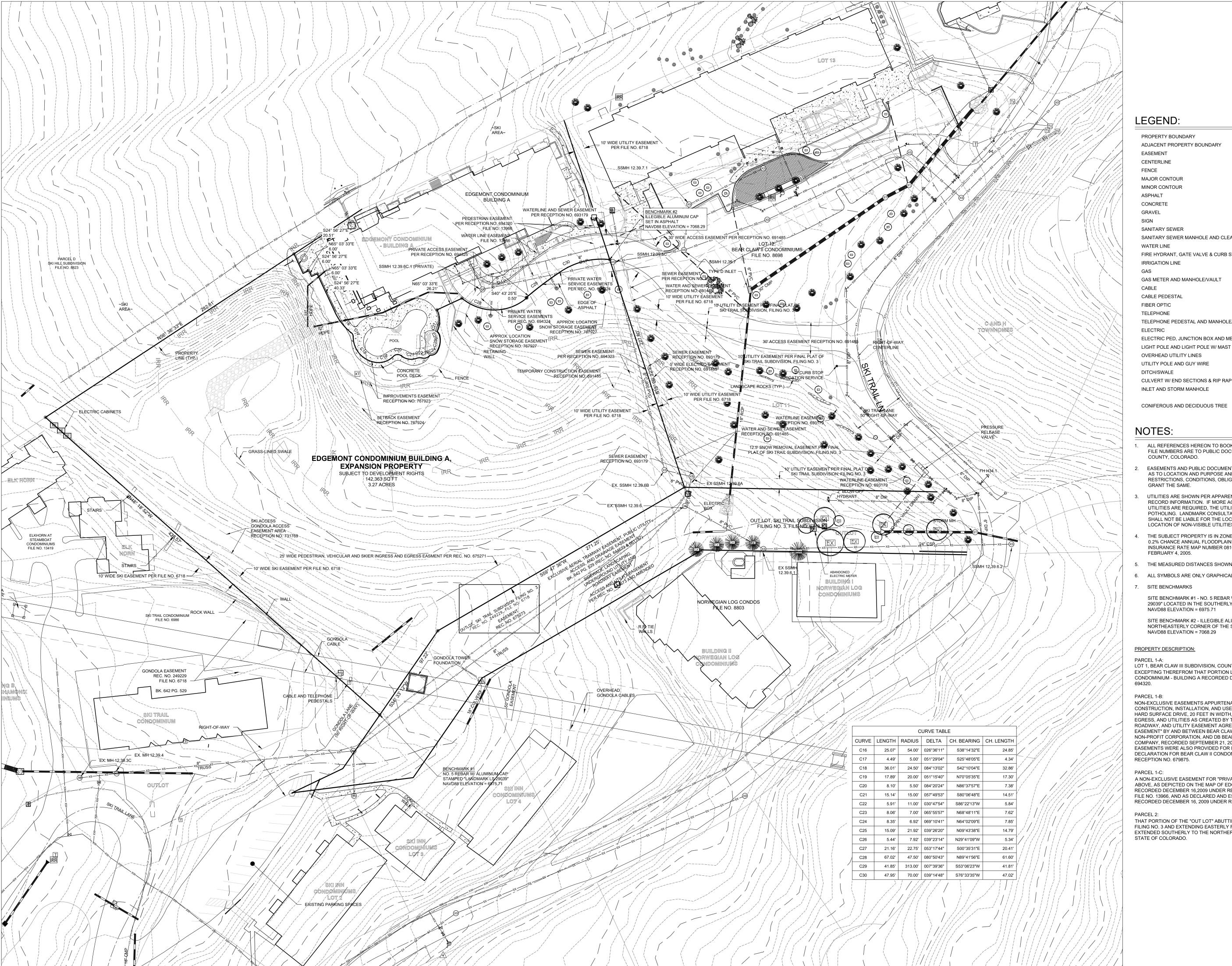
PROPERTY BOUNDARY ADJACENT PROPERTY BOUNDARY SANITARY SEWER MANHOLE AND CLEANOUT FIRE HYDRANT, GATE VALVE & CURB STOP GAS METER AND MANHOLE/VAULT TELEPHONE PEDESTAL AND MANHOLE/VAULT EJ ELECTRIC PED, JUNCTION BOX AND METER LIGHT POLE AND LIGHT POLE W/ MAST **♦** ★ OVERHEAD UTILITY LINES UTILITY POLE AND GUY WIRE
