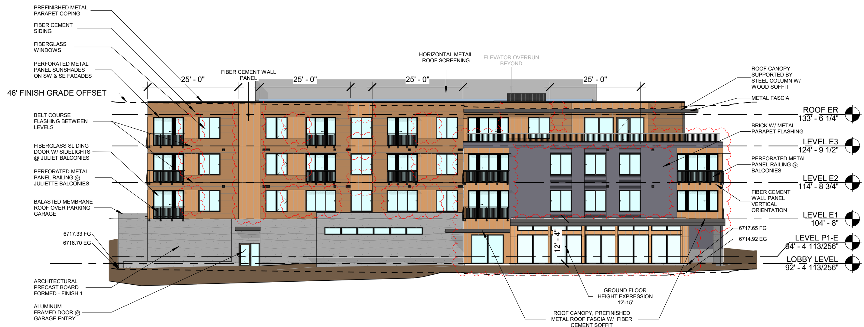
3 LOT E - SOUTH-WEST ELEVATION (REAR) SCALE: 1/16" = 1'-0"
