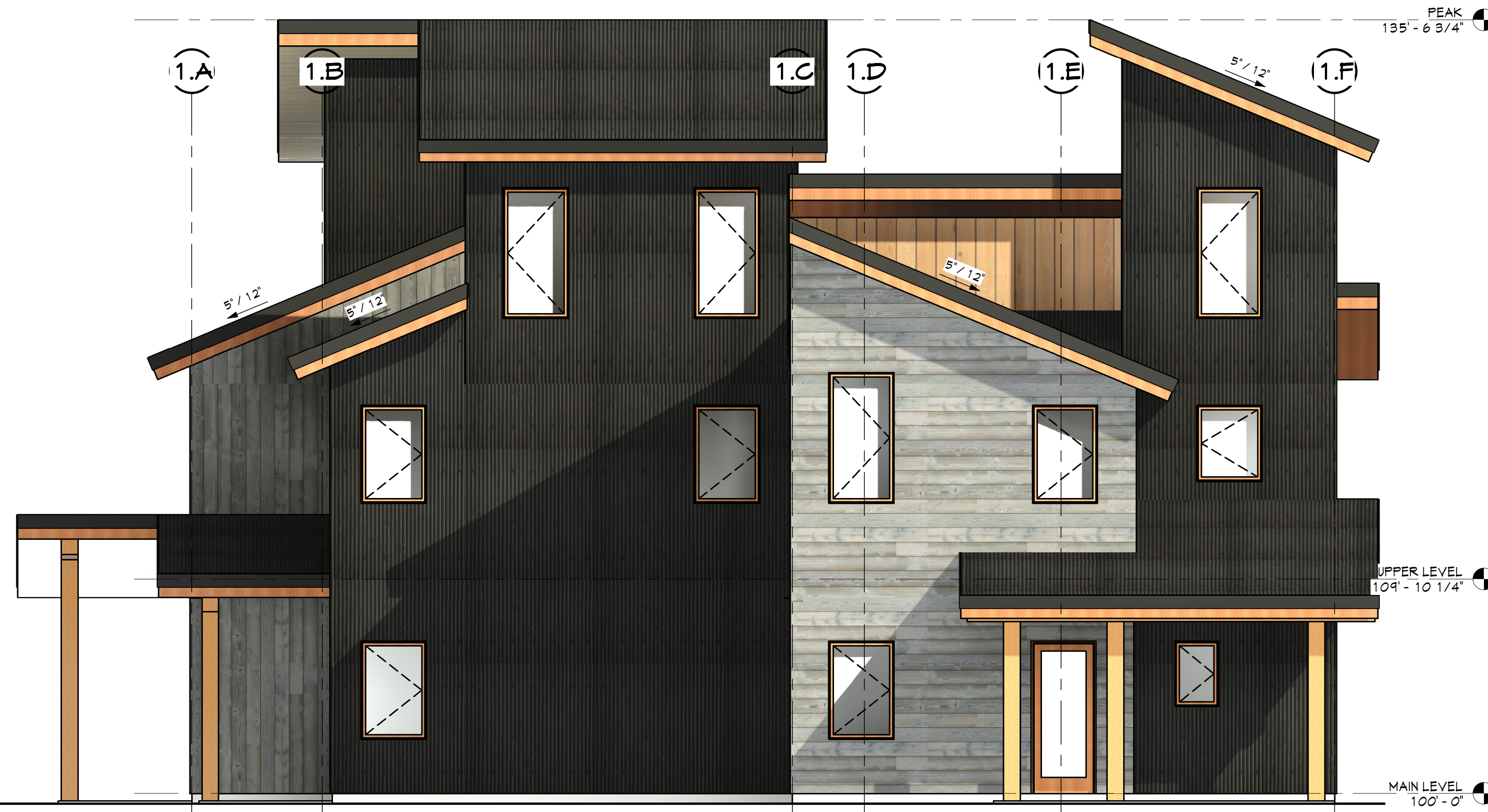
② Elevation BD 1 NORTHWEST 1/4" = 1'-0" (GLAZING = 12.8%)
