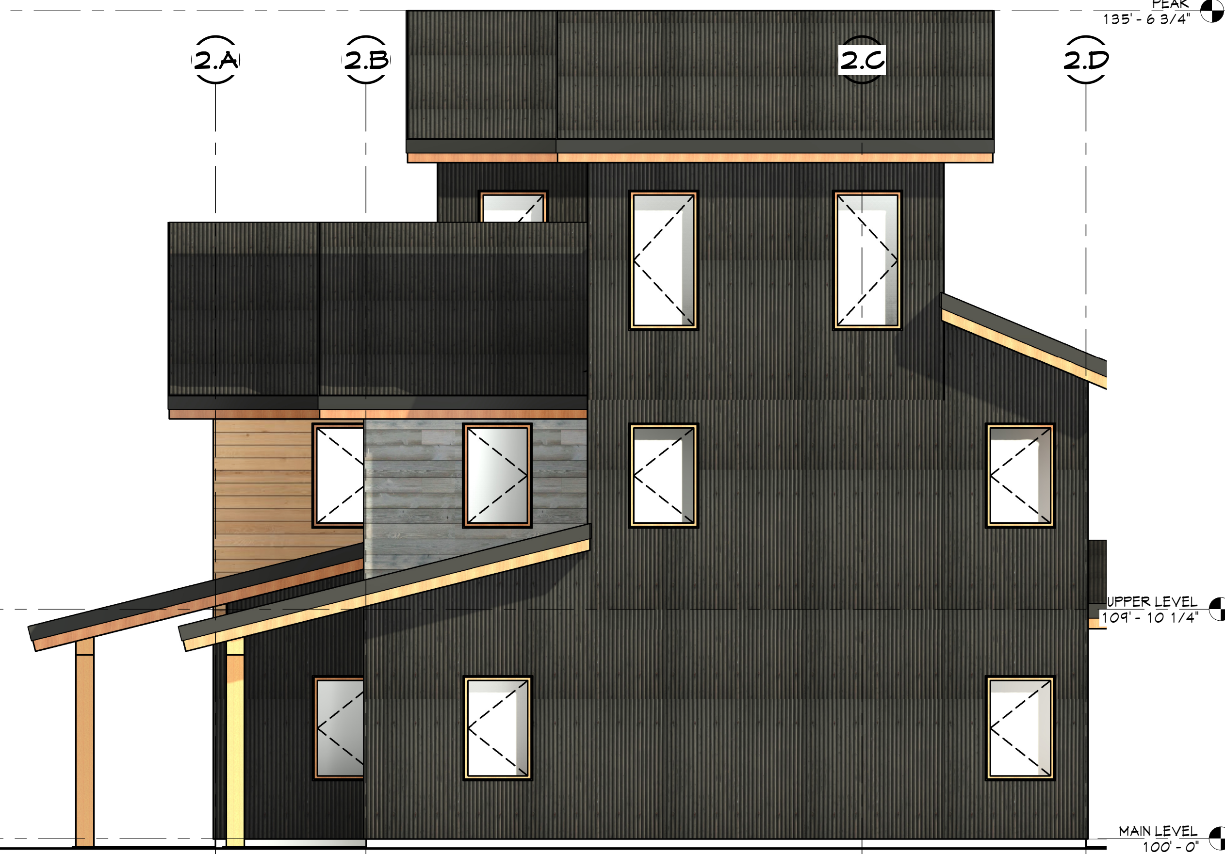
④ Elevation BD2 NORTHWEST 1/4" = 1'-0" (GLAZING = 14.2%)
