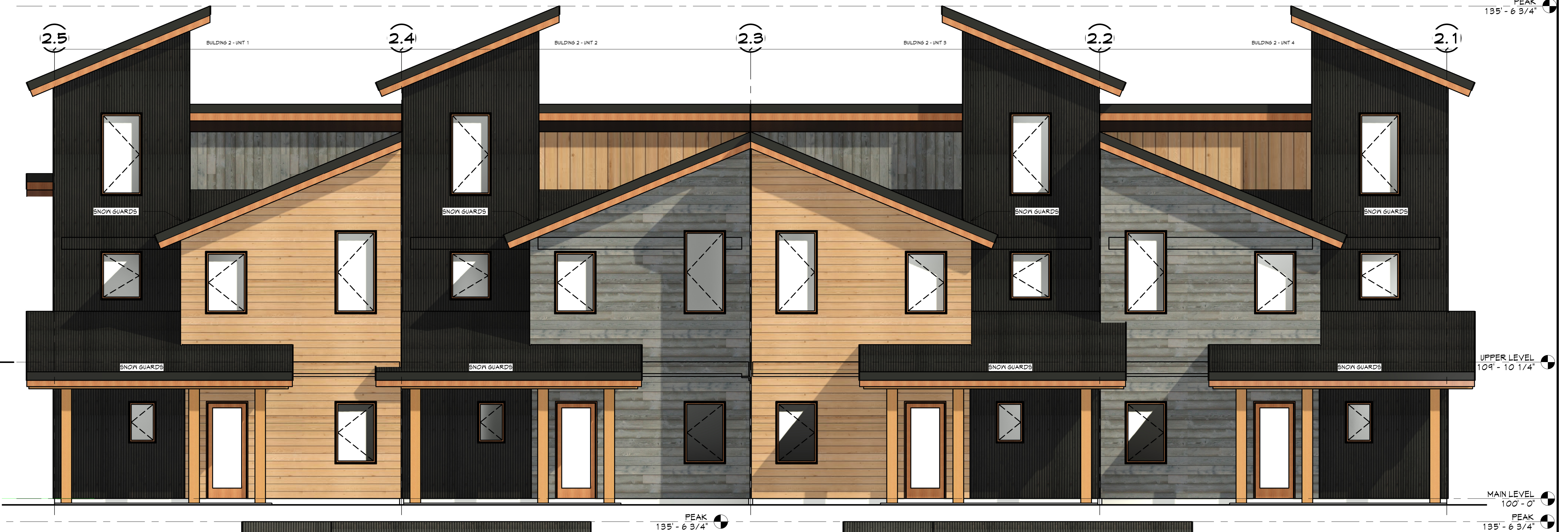
③ Elevation BD2 SOUTHWEST 1/4" = 1'-0" (GLAZING = 13.4%)
