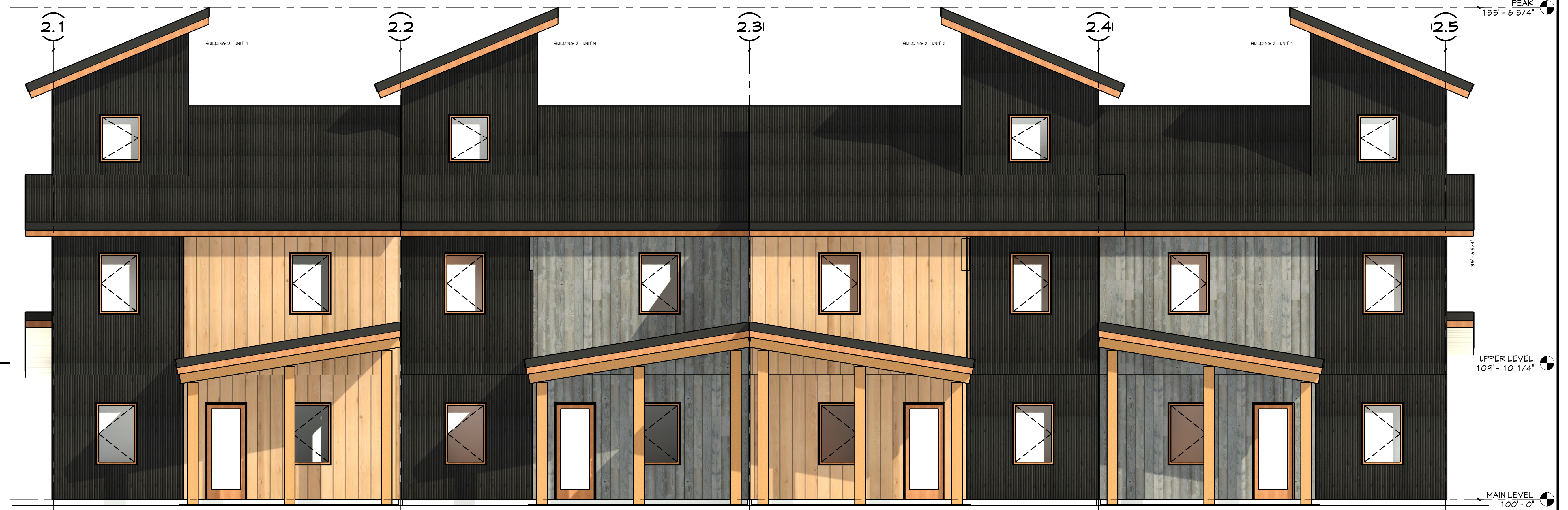
① Elevation BD2 NORTHEAST 1/4" = 1'-0" (GLAZING = 16.2%)
