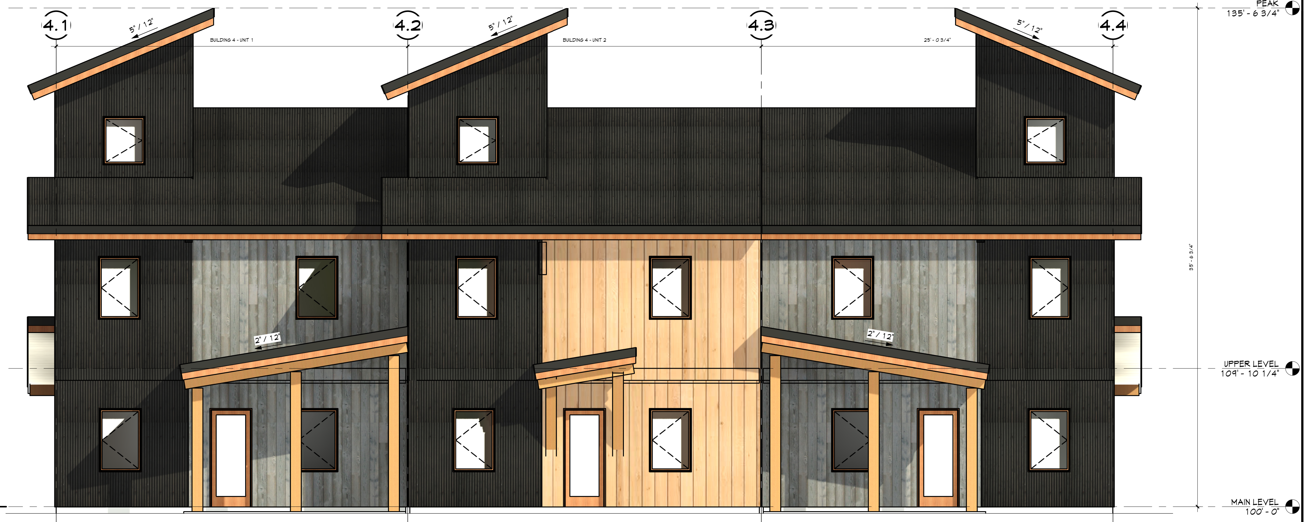
③ Elevation BD4 SOUTHEAST 1/4" = 1'-0" (GLAZING = 16.2%)
