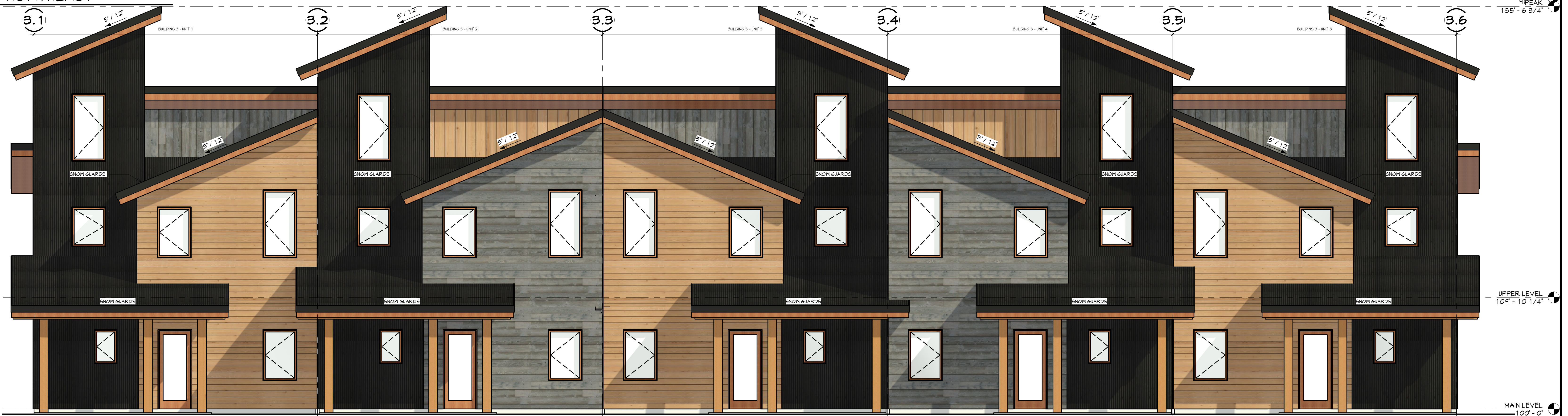
④ Elevation BD3 SOUTHWEST 1/4" = 1'-0" (GLAZING = 13.4%)
