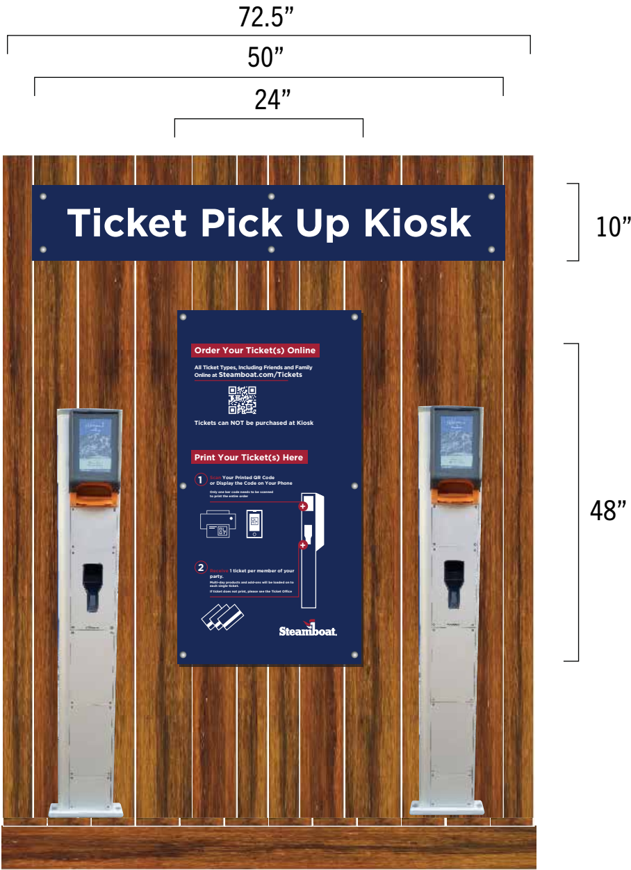
24 FS-11 & FS-12 : Ticket Pickup Kiosk - Double Version SP-4, J11 & R3 Current drawings represent 2 double kiosks. Maximum allowance is 5
