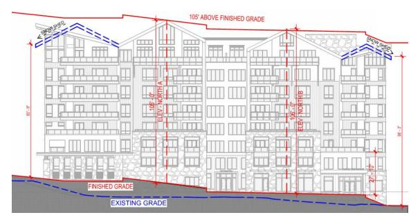
Snow fences, snow clips, and snow melt can be provided in these locations, but this does not guarantee the catchment of all snow from falling to the pedestrian paths below. The proposed design with a 3:12 slope away from the pedestrian paths is the best solution.
