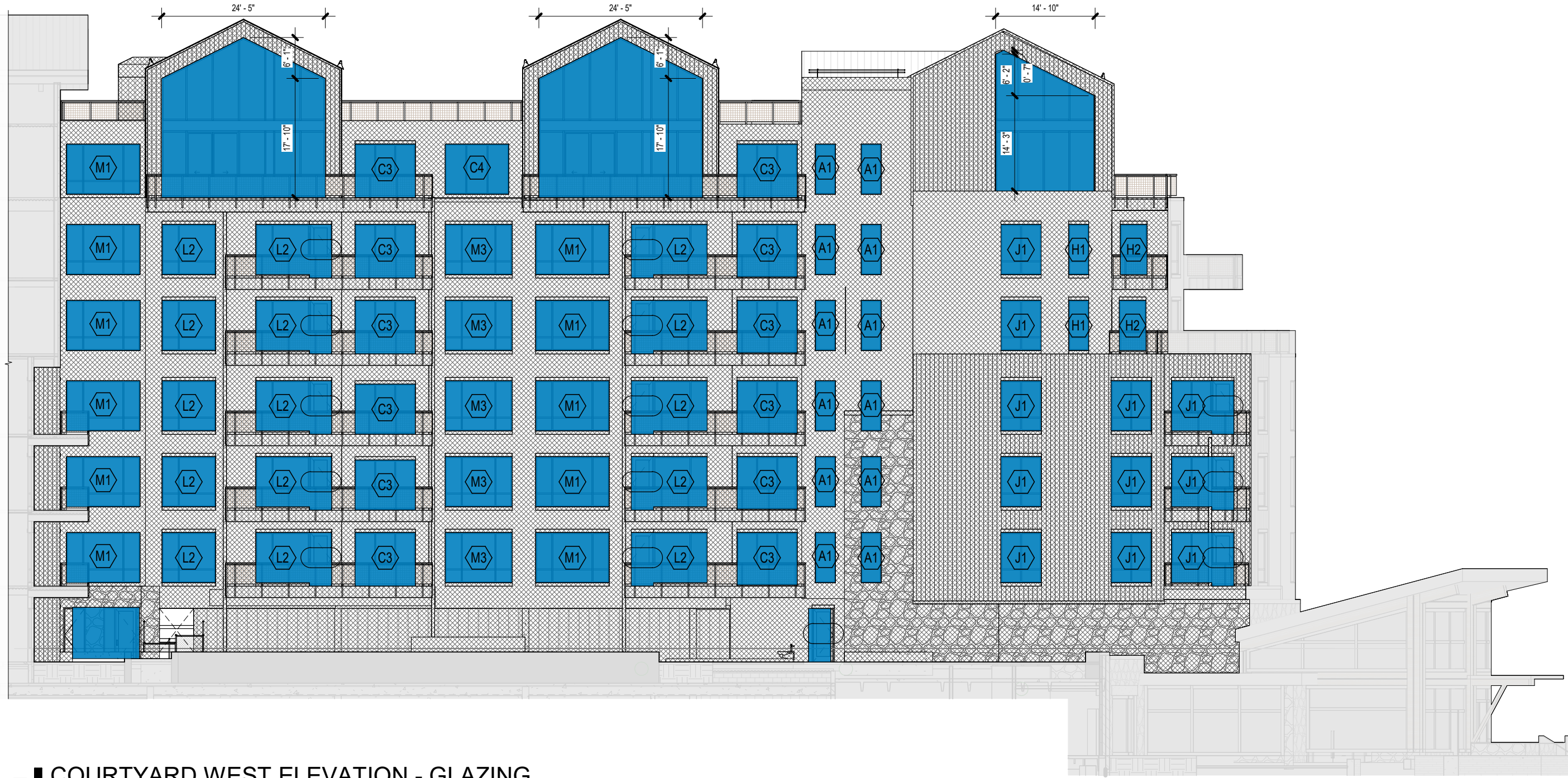
5 | COURTYARD WEST ELEVATION - GLAZING 1/16" = 1'-0"
