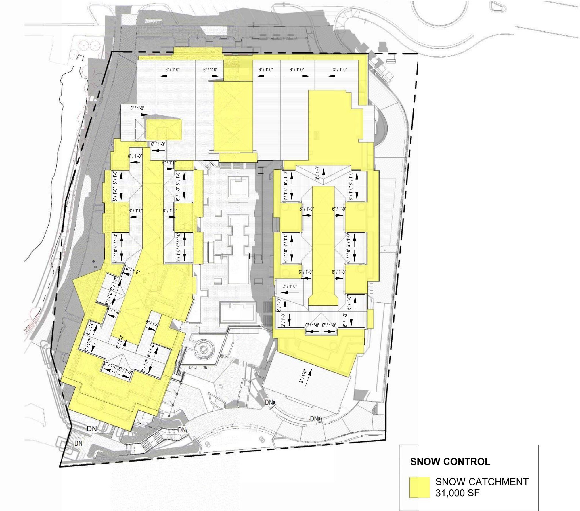
3 ROOF PLAN - SNOW RETENTION & CONTROL 1" = 50'-0"
