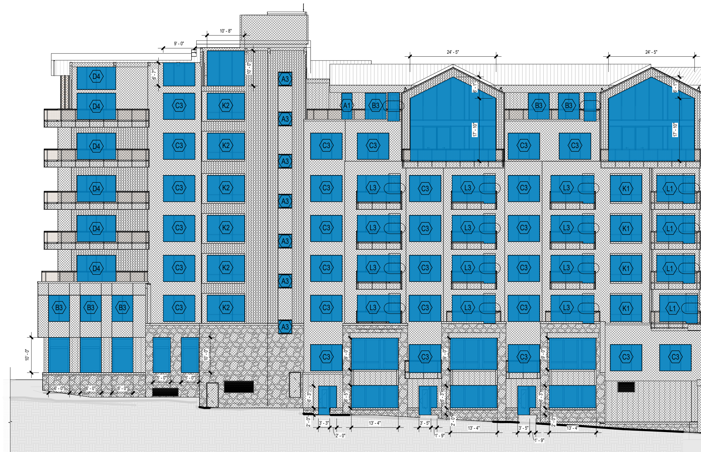
2 WEST BUILDING ELEVATION - NORTH SIDE - GLAZING 1/16" = 1'-0"
