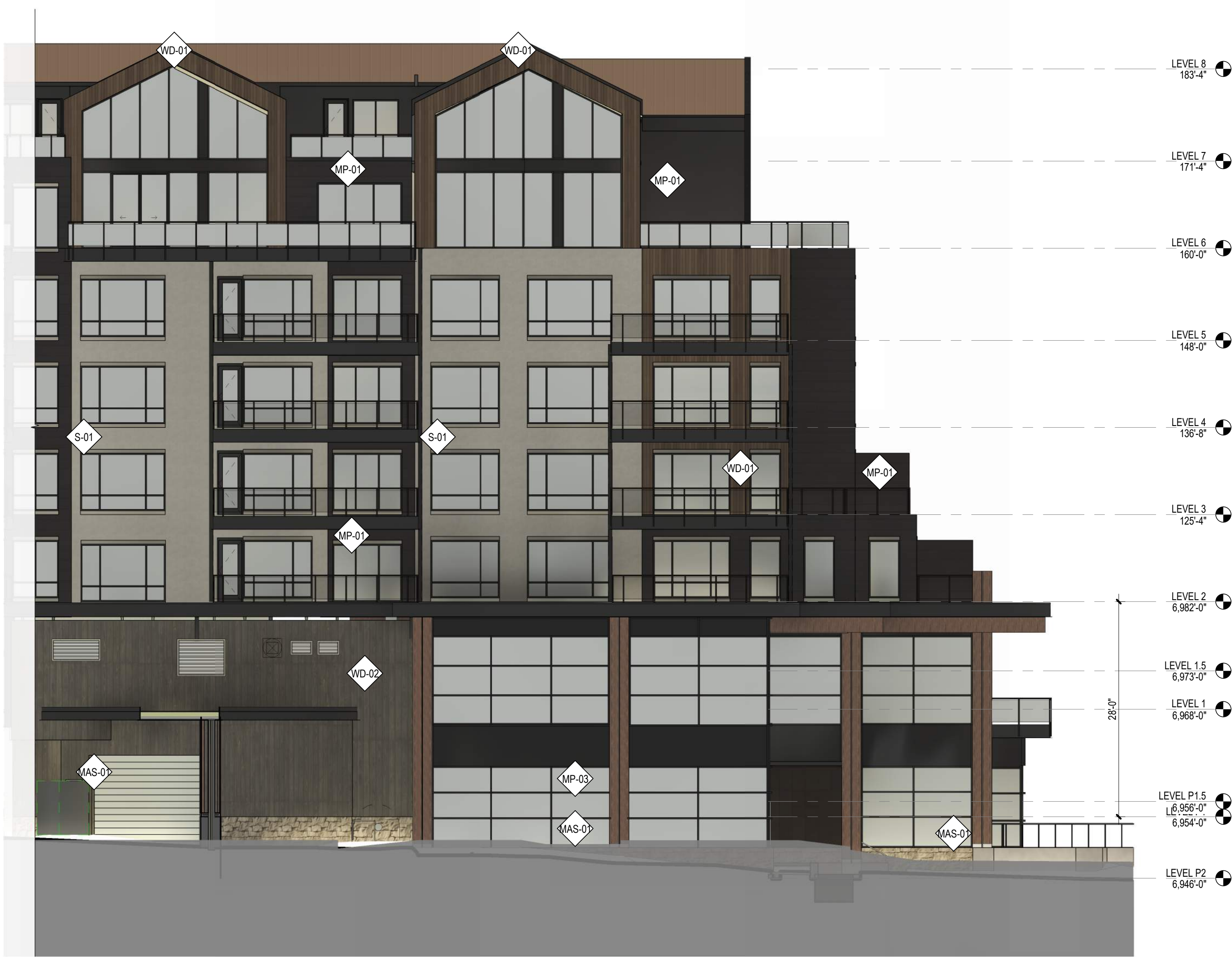
2 WEST BUILDING ELEVATION - SOUTH SIDE 3/32" = 1'-0"
