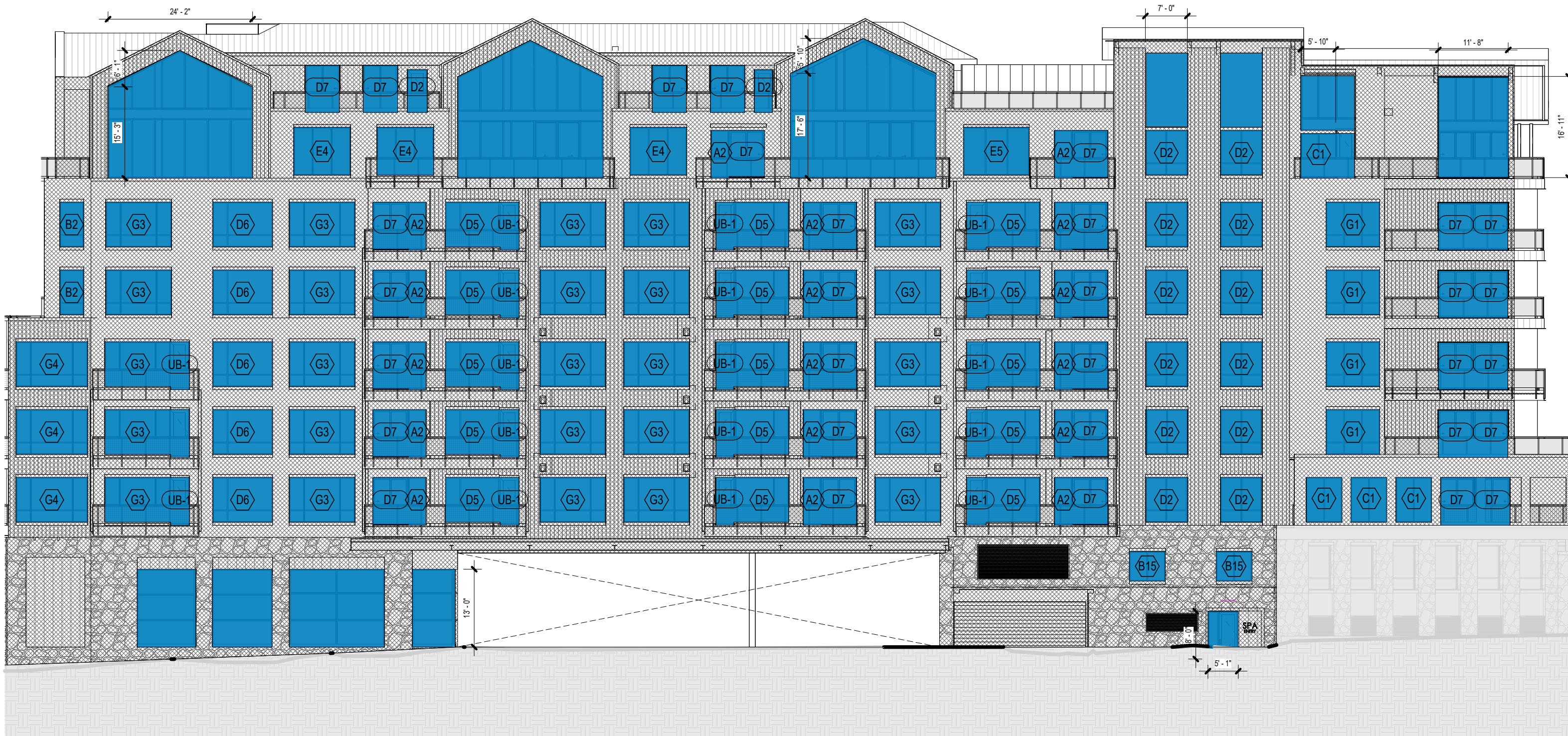
4 EAST OVERALL BUILDING ELEVATION - GLAZING 1/16" = 1'-0"
