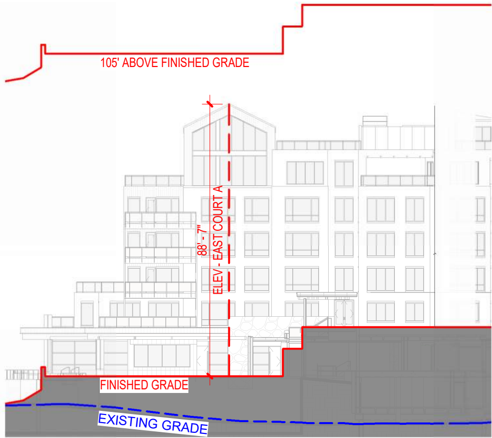
9 | LOWER COURTYARD EAST ELEVATION - HEIGHT 1/32" = 1'-0"
