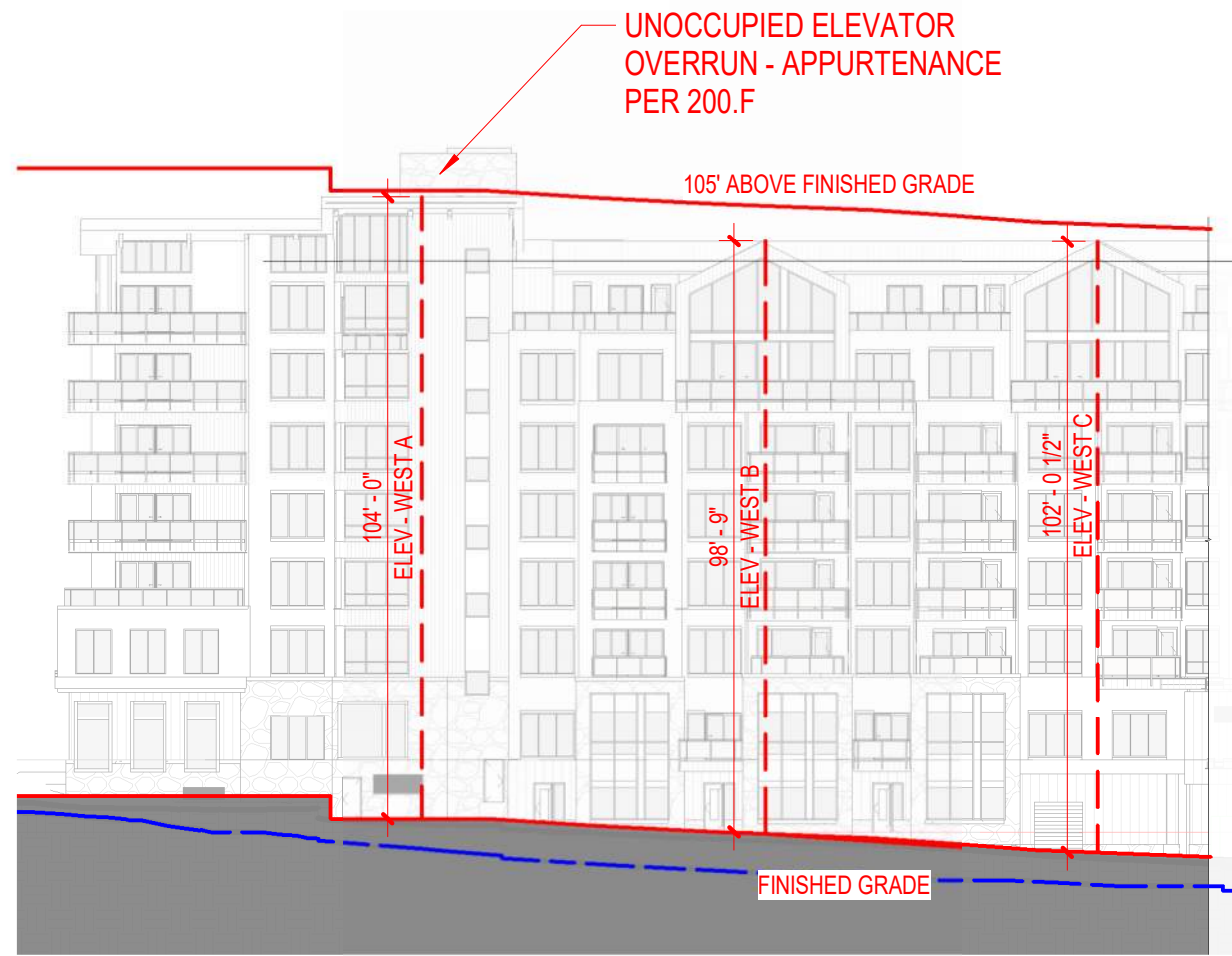
3 | WEST ELEVATION - NORTH SIDE - HEIGHT 1/32" = 1'-0"
