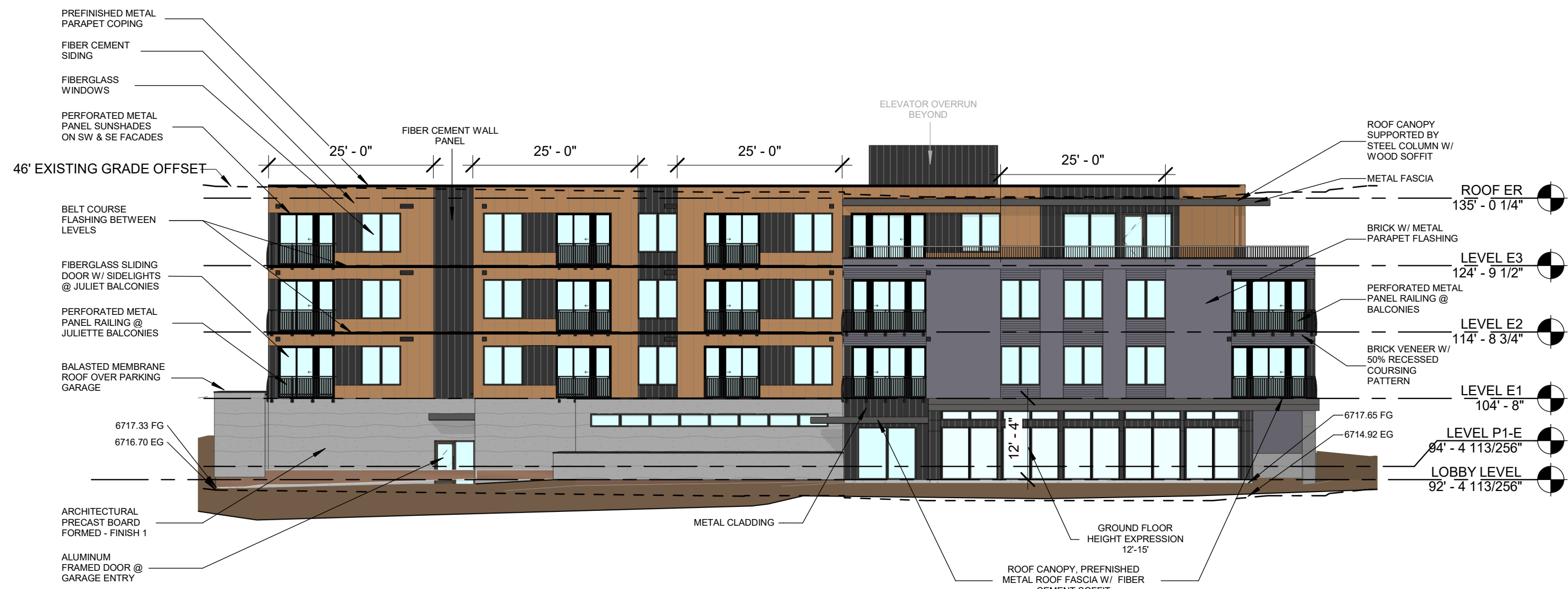
3 LOT E - SOUTH-WEST ELEVATION (REAR) SCALE: 1/16" = 1'-0"
