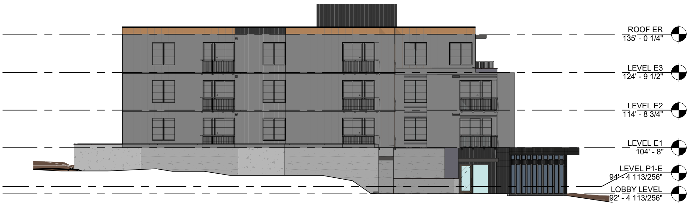
LOT E - NORTH-WEST ELEVATION (SIDE) SD Copy 1 SCALE: 1/16" = 1'-0"
