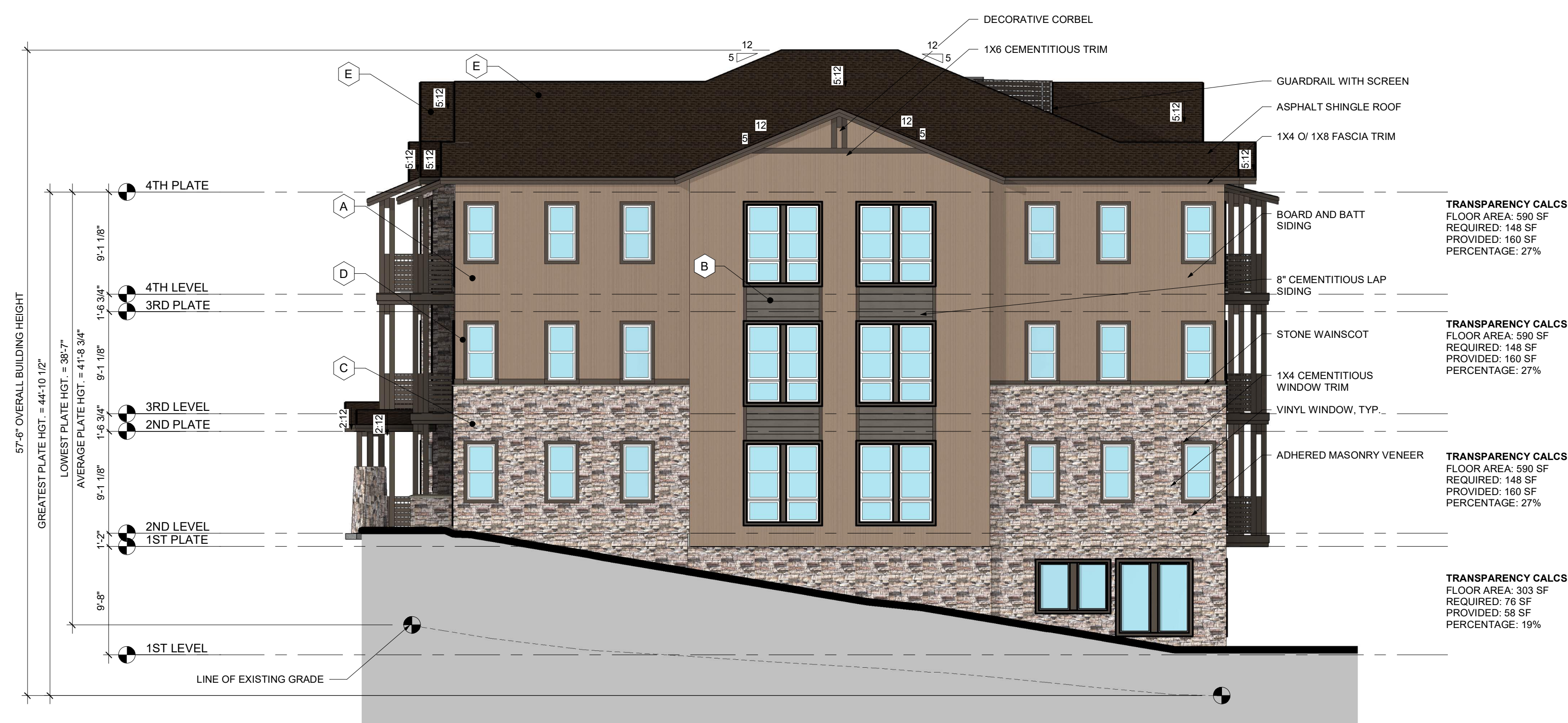
1 BUILDING 3 (TYPE 1A) - REAR ELEVATION 1/8" = 1'-0"
