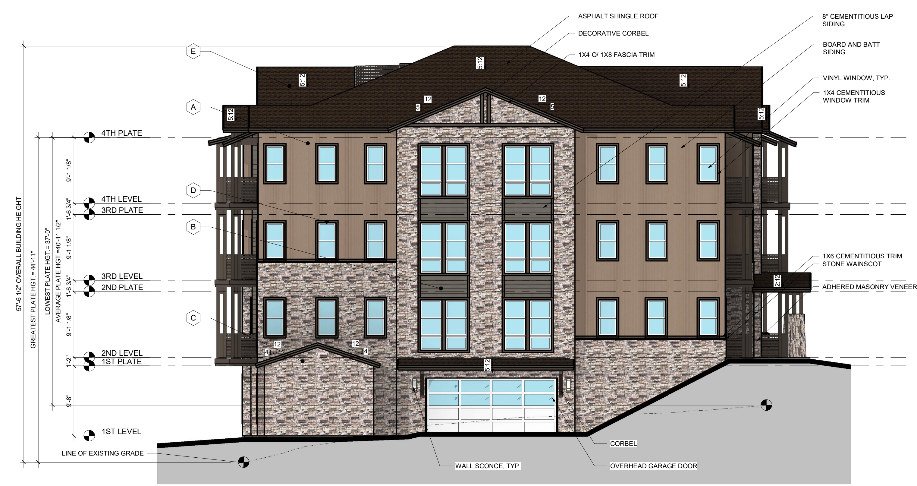
1 BUILDING 3 (TYPE 1A) - FRONT ELEVATION 1/8" = 1'-0"
