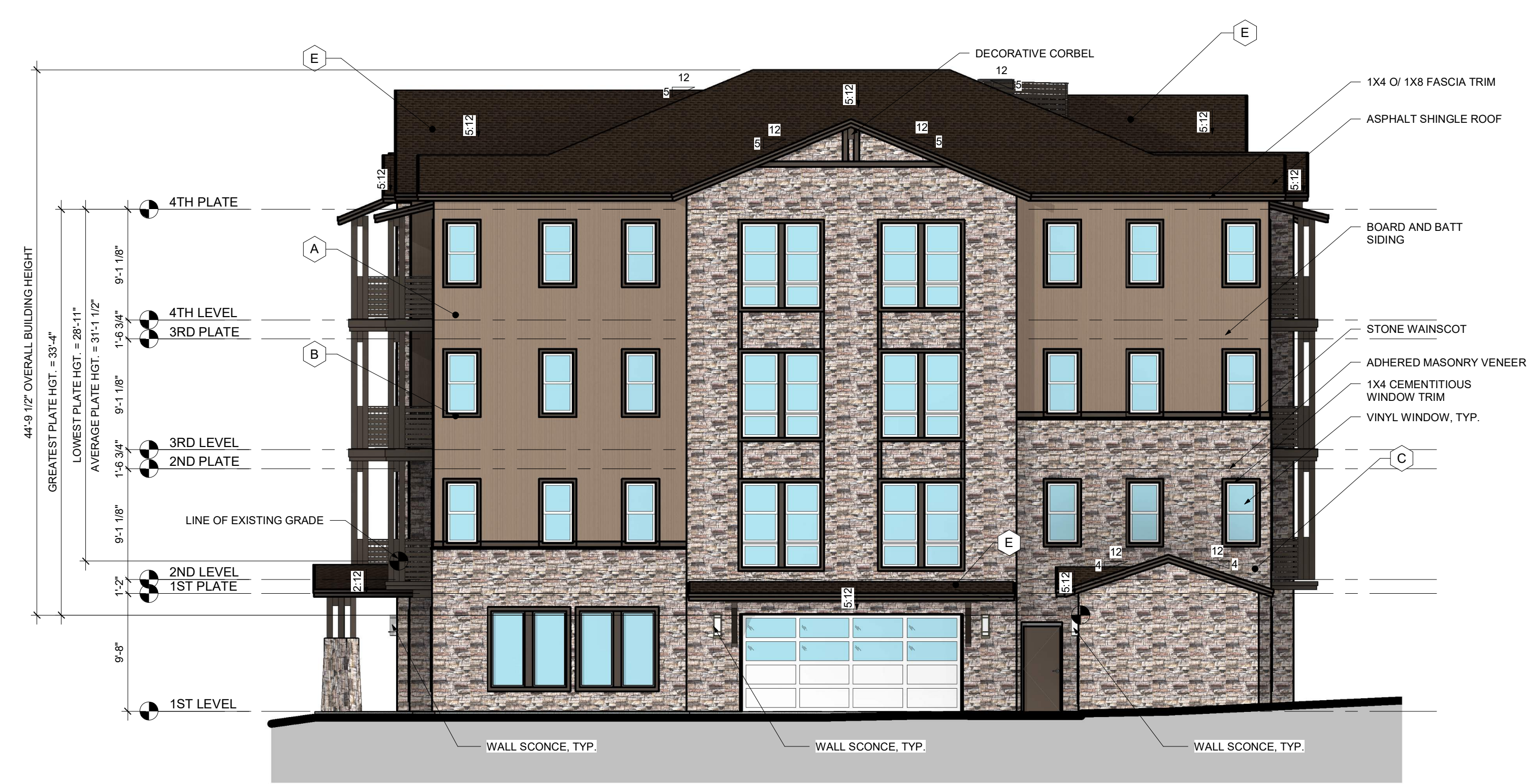
1 BUILDING 7 (TYPE 2) - REAR ELEVATION 1/8" = 1'-0"
