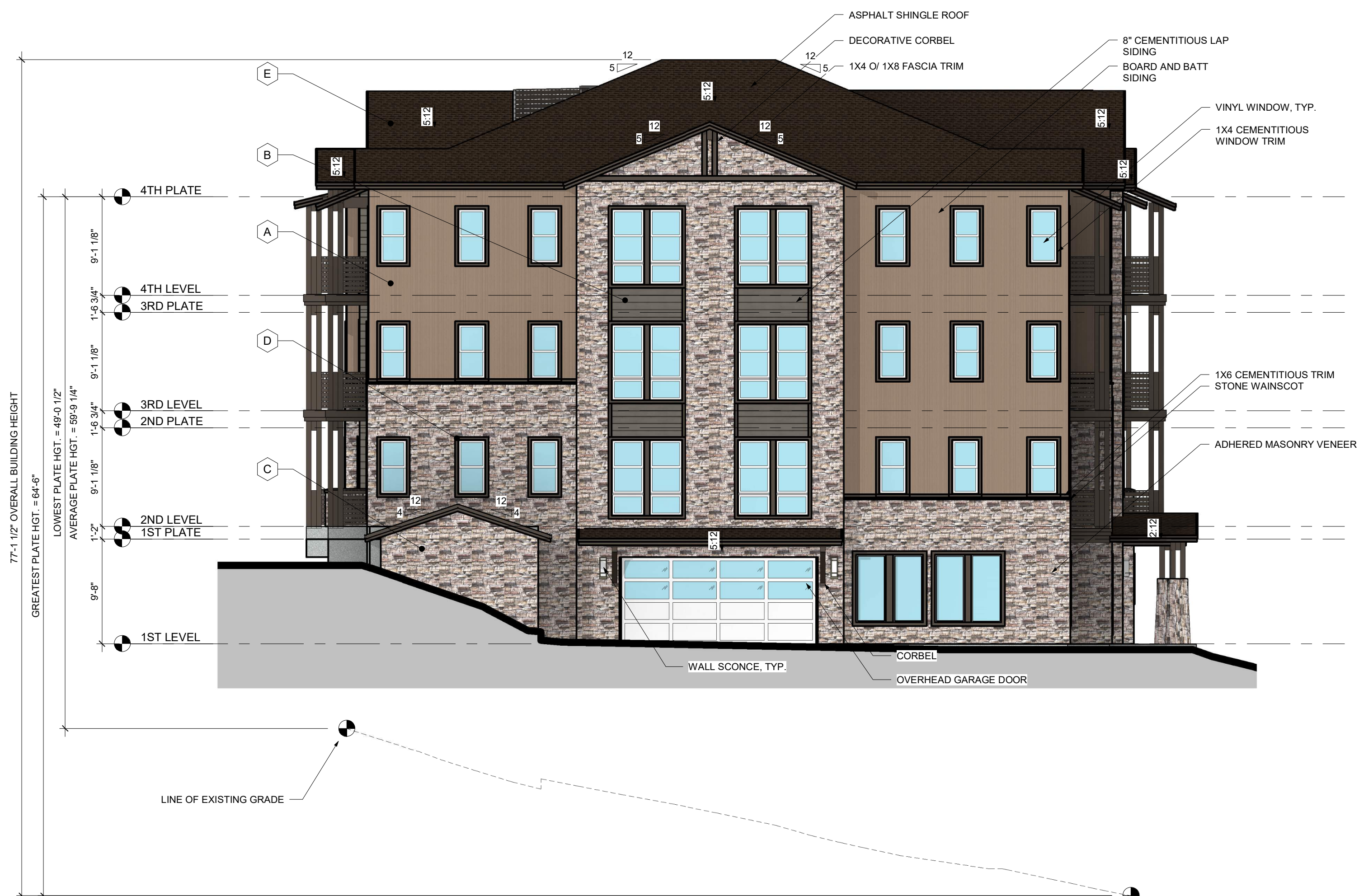
2 BUILDING 5 (TYPE 1A) - LEFT ELEVATION 1/8" = 1'-0"
