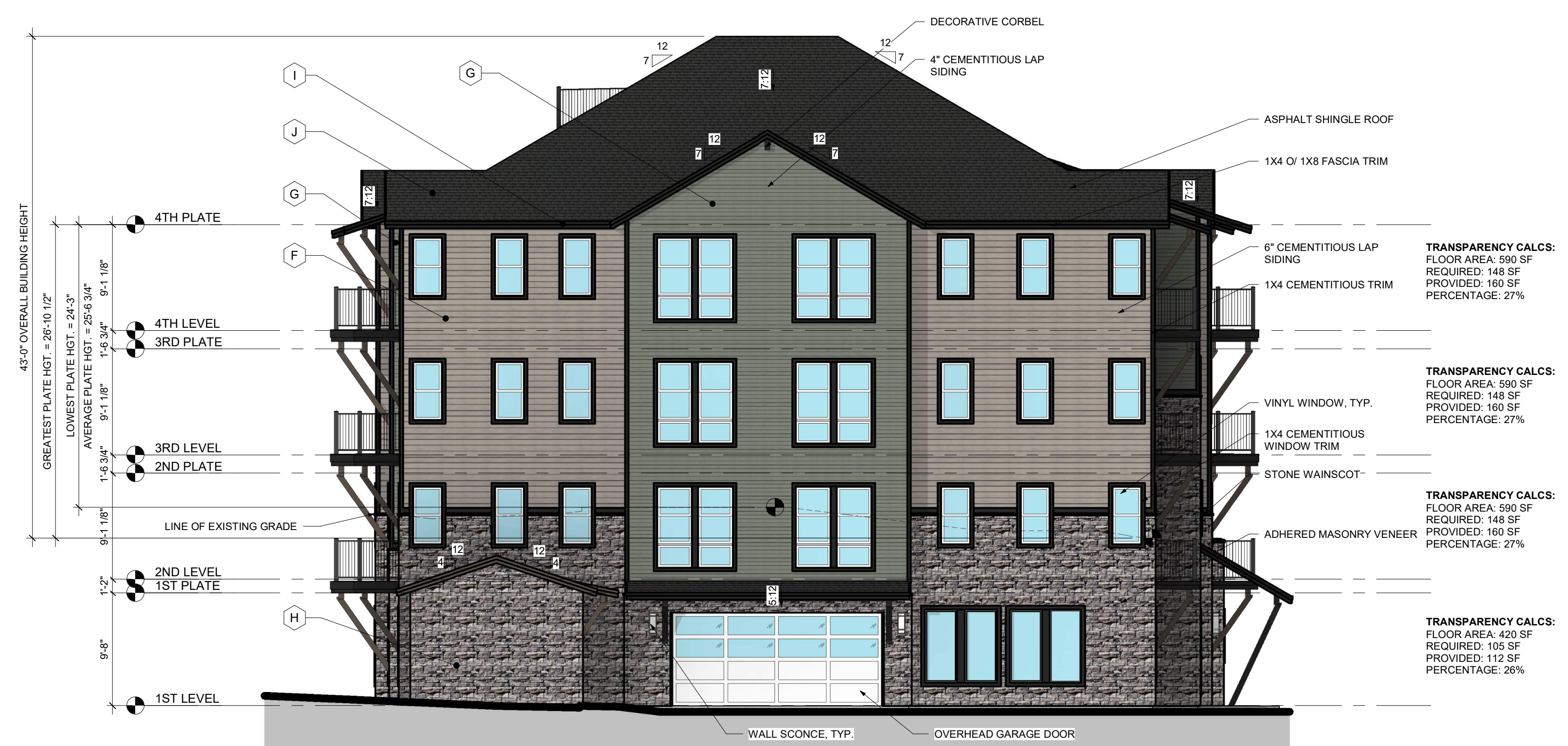
1 BUILDING 6 (TYPE 1B) - FRONT ELEVATION 1/8" = 1'-0"
