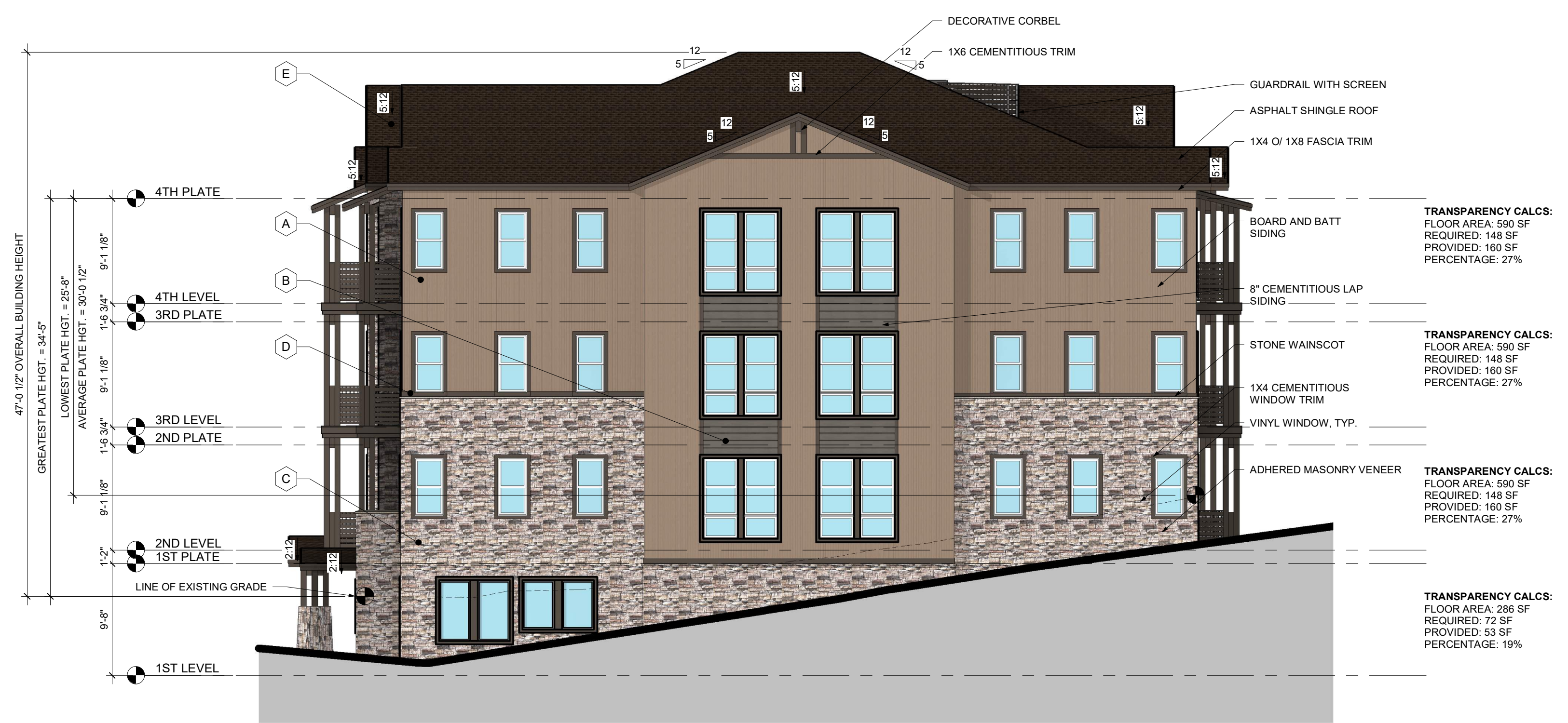
1 BUILDING 5 (TYPE 1A) - REAR ELEVATION 1/8" = 1'-0"
