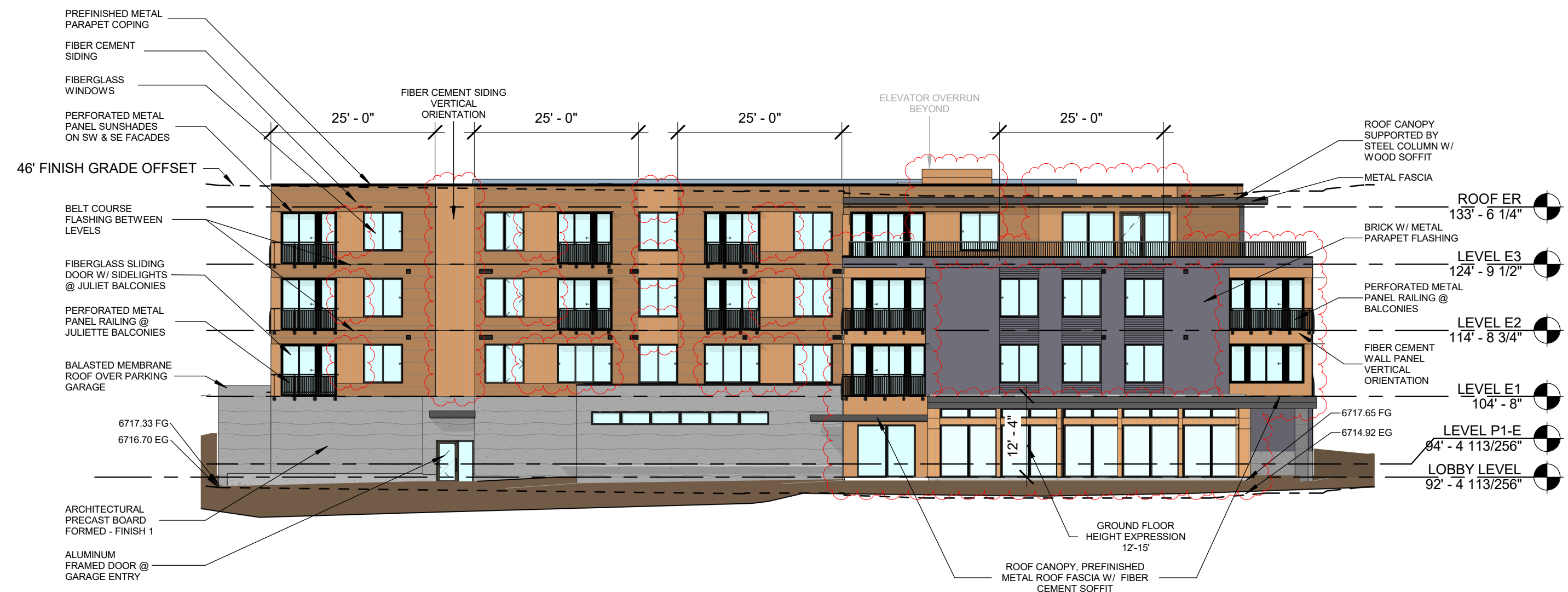
3 LOT E - SOUTH-WEST ELEVATION (REAR) SCALE: 1/16" = 1'-0"
