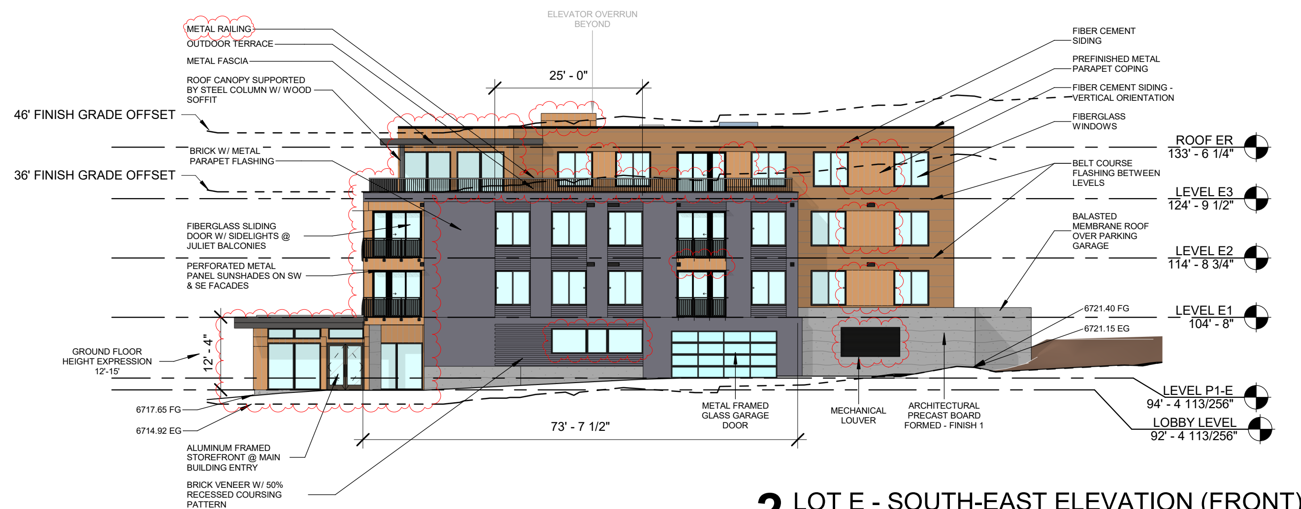
2 LOT E - SOUTH-EAST ELEVATION (FRONT) SCALE: 1/16" = 1'-0"
