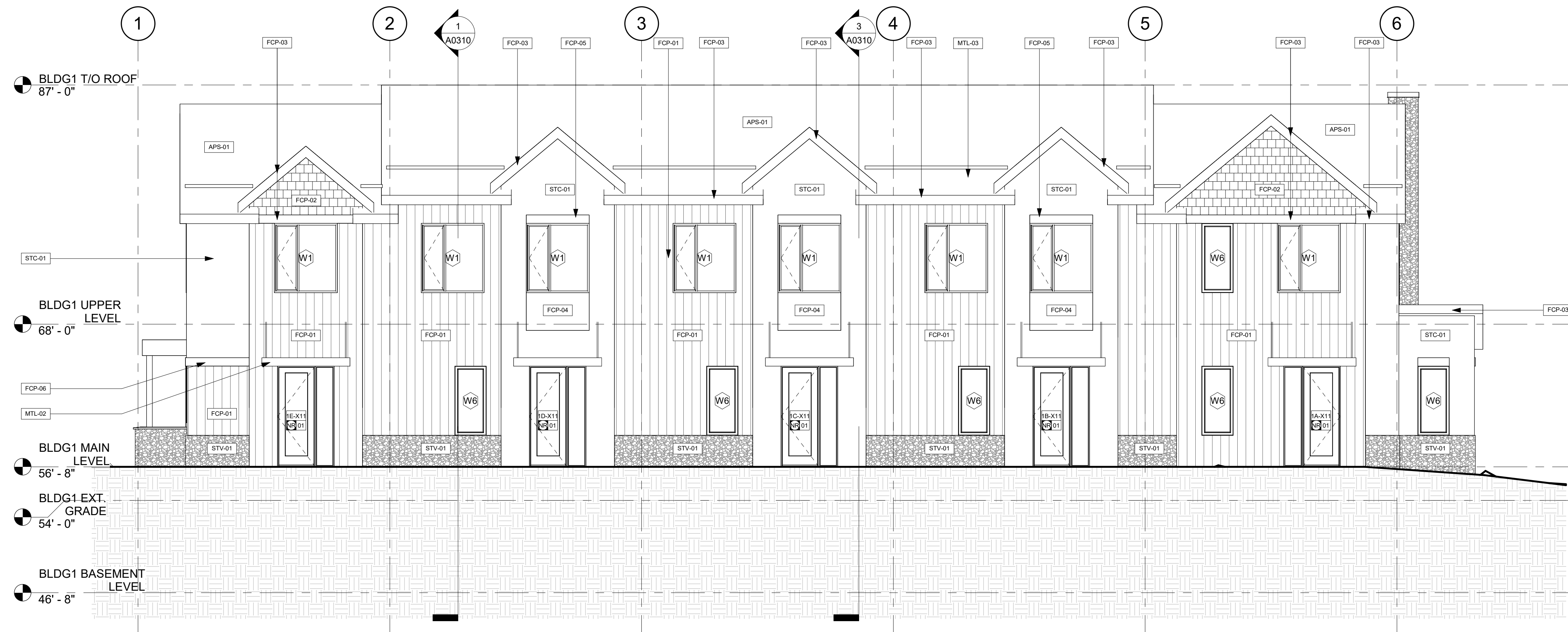
2 BLDG 1 EAST ELEVATION A0200A0300 3/16" = 1'-0"
