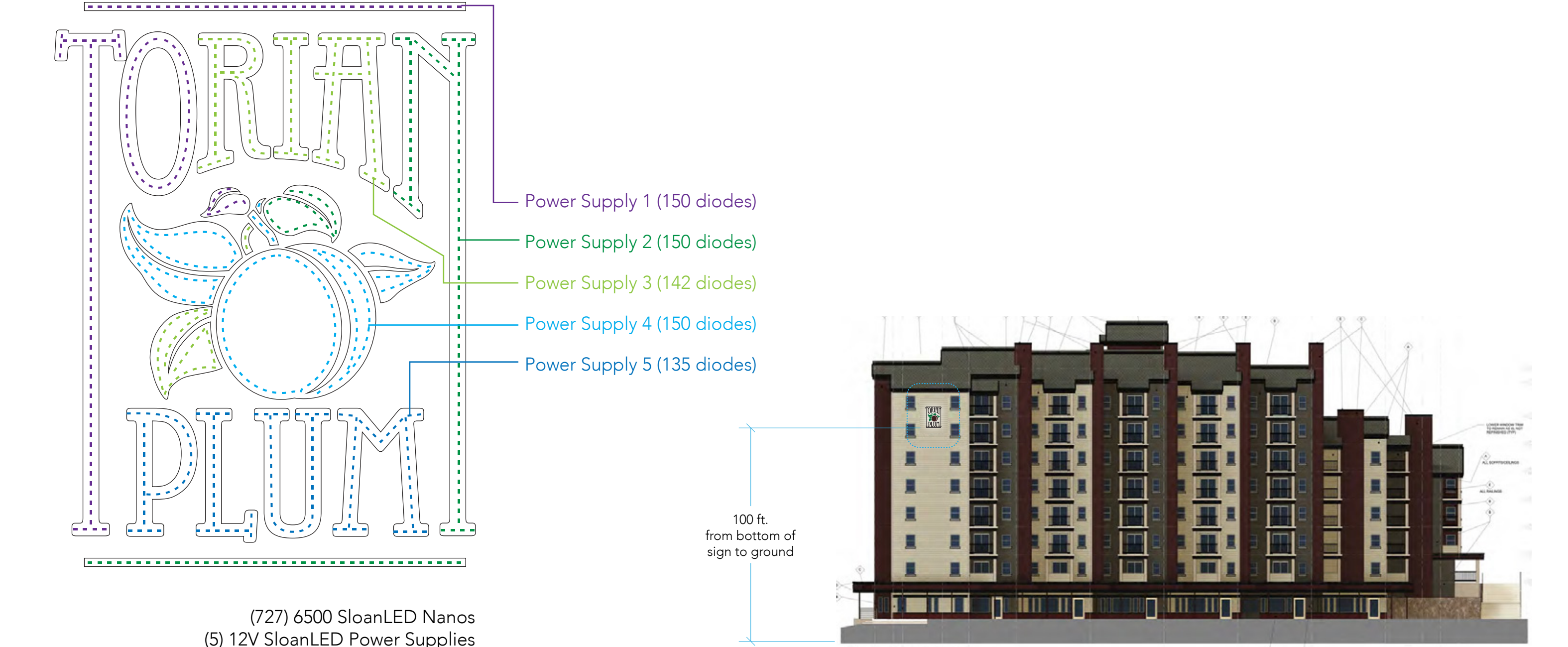
D> LED Light Layout 1:15 scale E> Building A&B SOUTH Elevation scale: 1/8" = 4'
