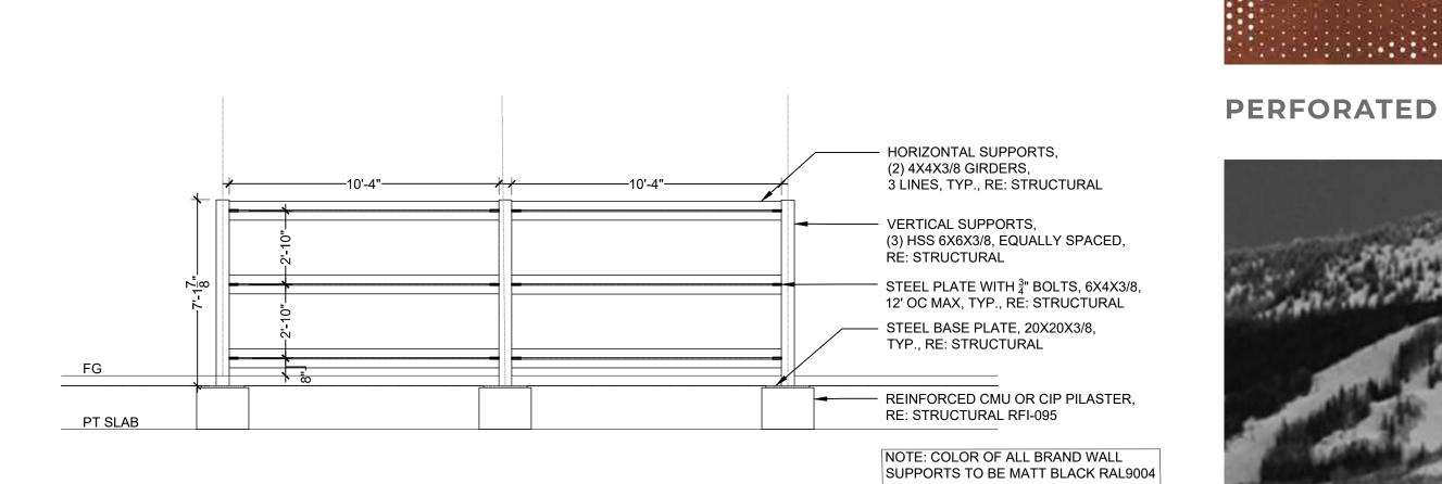
BRAND WALL STRUCTURAL SUPPORT ELEVATION
