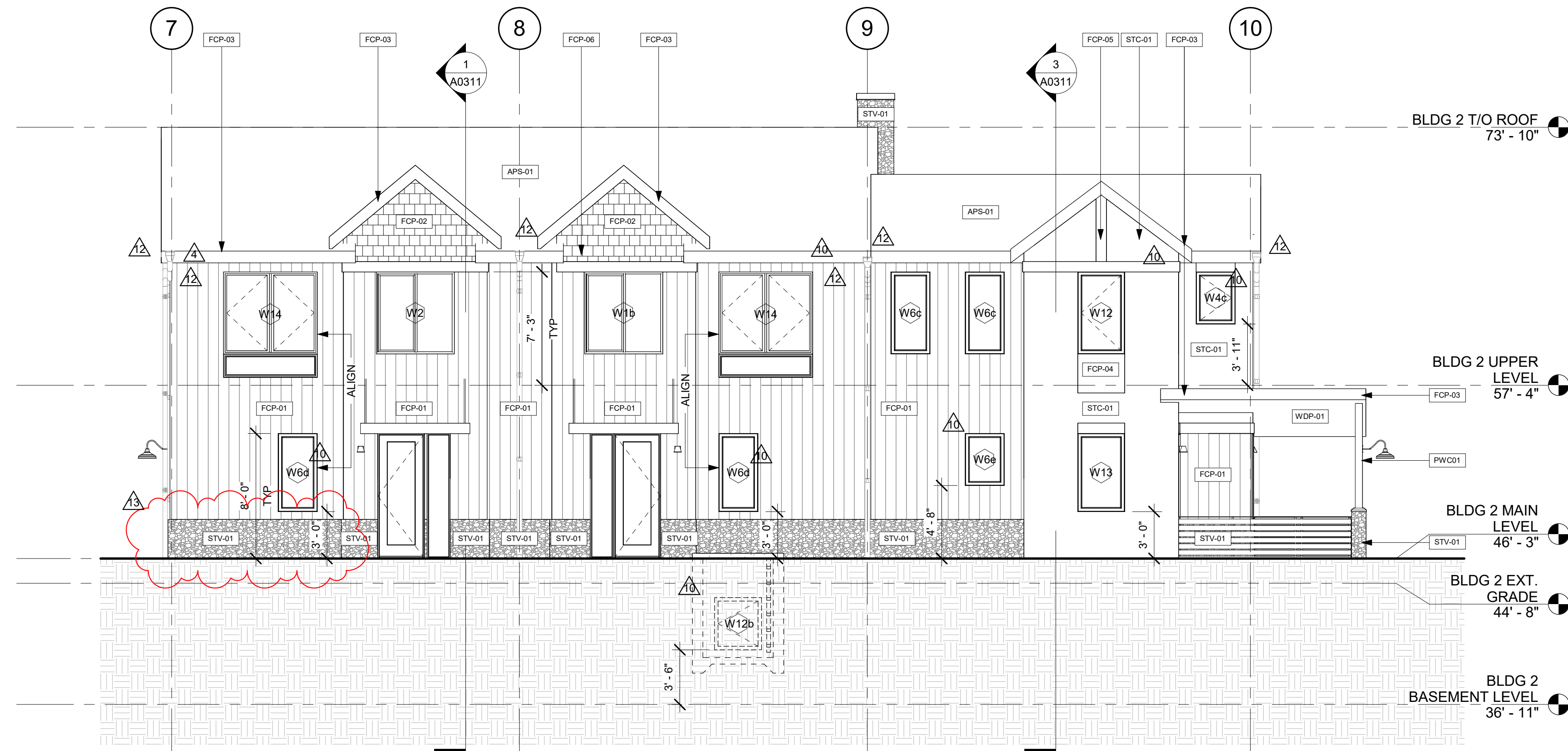
2 2075 EAST ELEVATION A0302/A0302 3/16" = 1'-0"
