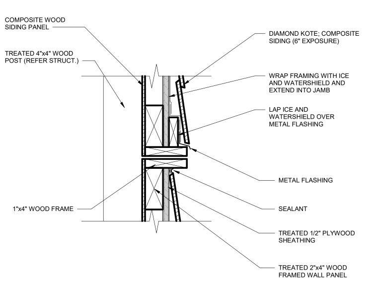
FRAMED DOOR PANEL COMPOSITE WOOD SIDING PANEL TREATED 4x4 WOOD POST BEYOND -STONE PAVERS ON CONCRETE SLAB —
