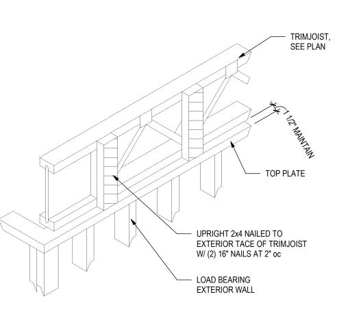
TRIM JOIST FLUSH PARALLEL TO EXT WALL S5.4 3/4" = 1'-0"
