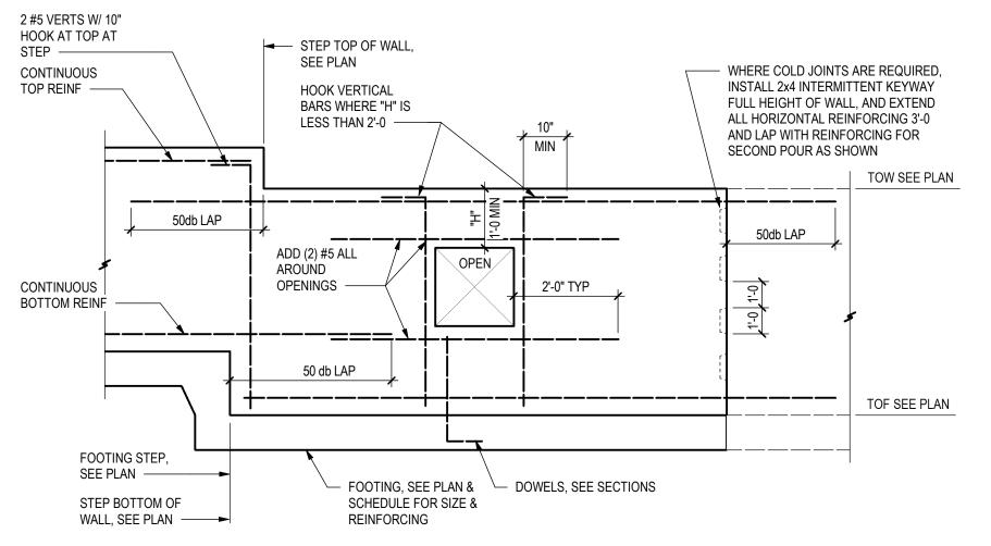
TYP WALL REINFORCEMENT AT STEPS & OPENINGS
