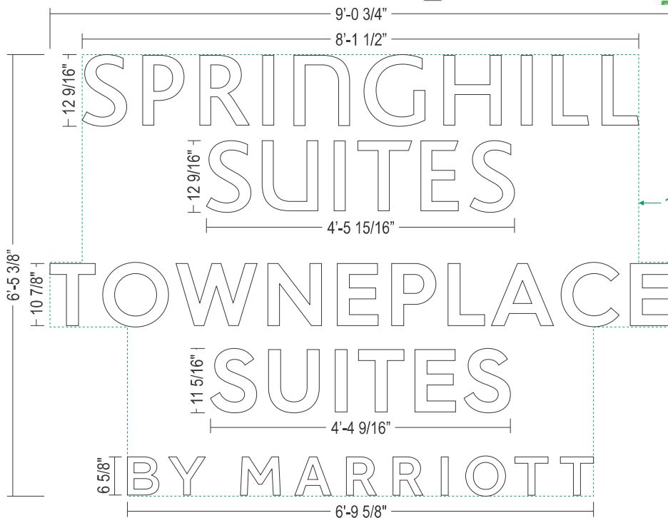
CUSTOM CHANNEL LETTER DETAILS SCALE: 1/2" = 1'-0"
