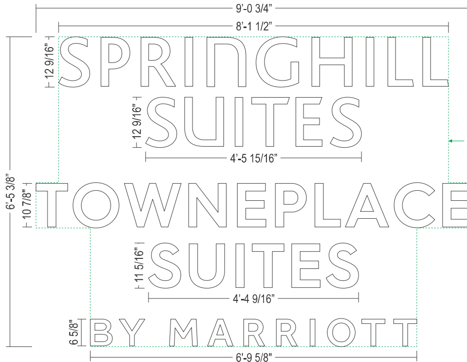
CUSTOM CHANNEL LETTER DETAILS SCALE: 1/2" = 1'-0"
