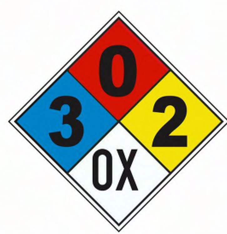
PLACECARD INFORMATION MAY DIFFER; REFER TO MSDS FROM PRODUCT MANUFACTURER NFPA PLACECARD CALCIUM HYPOCHLORITE 2 NO SCALE
