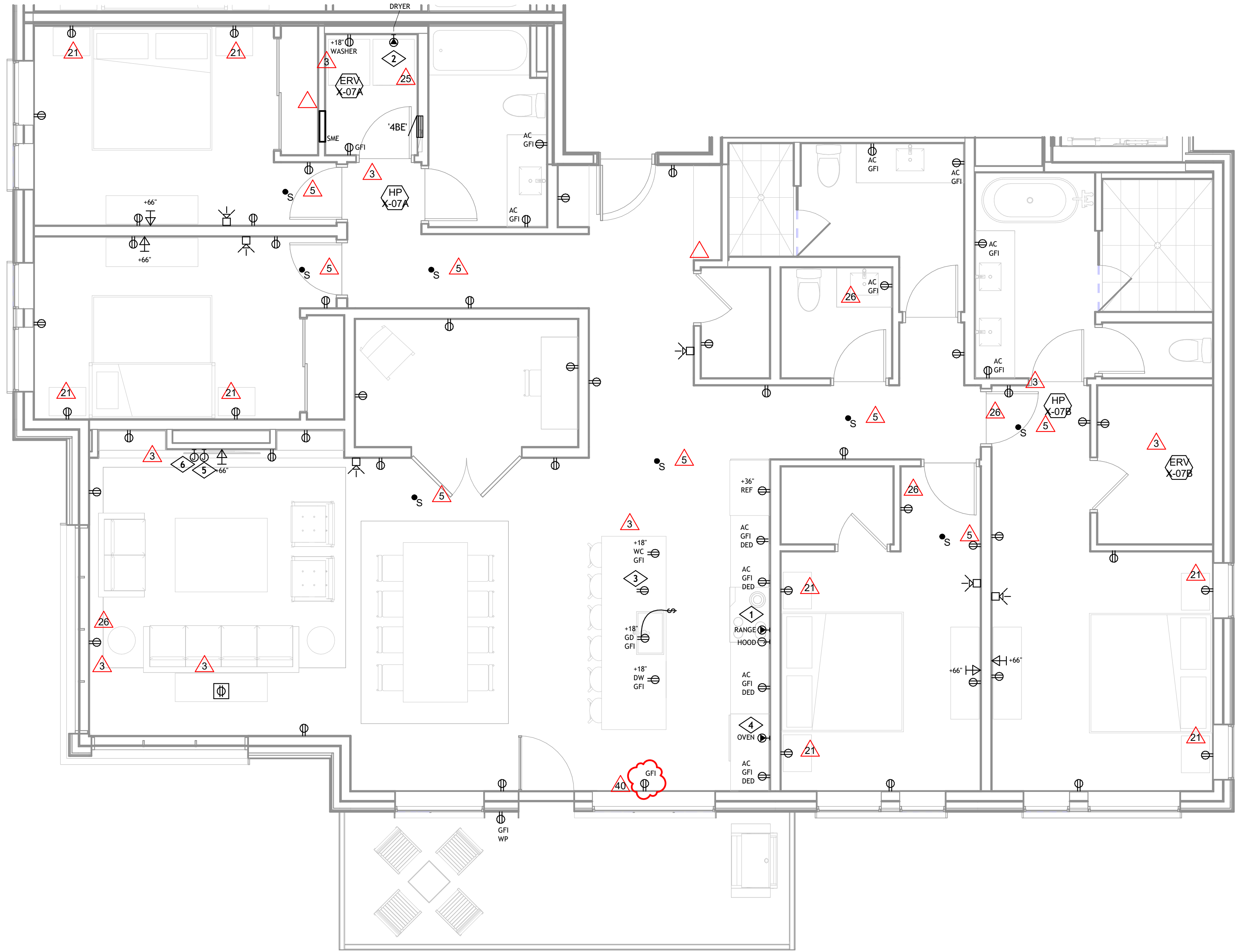
1 | ELECTRICAL POWER UNIT PLAN - 4 BEDROOM EAST LVL 2-4 E2.13 | 1/4" = 1'-0"
