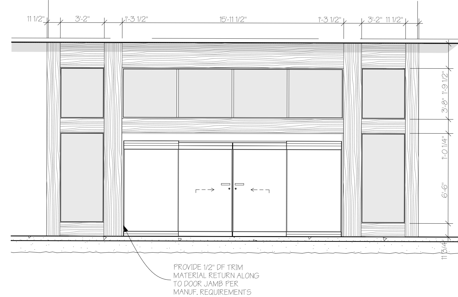
8 ENTRY INTERIOR ELEVATION SCALE: 1/4" = 1'-0"
