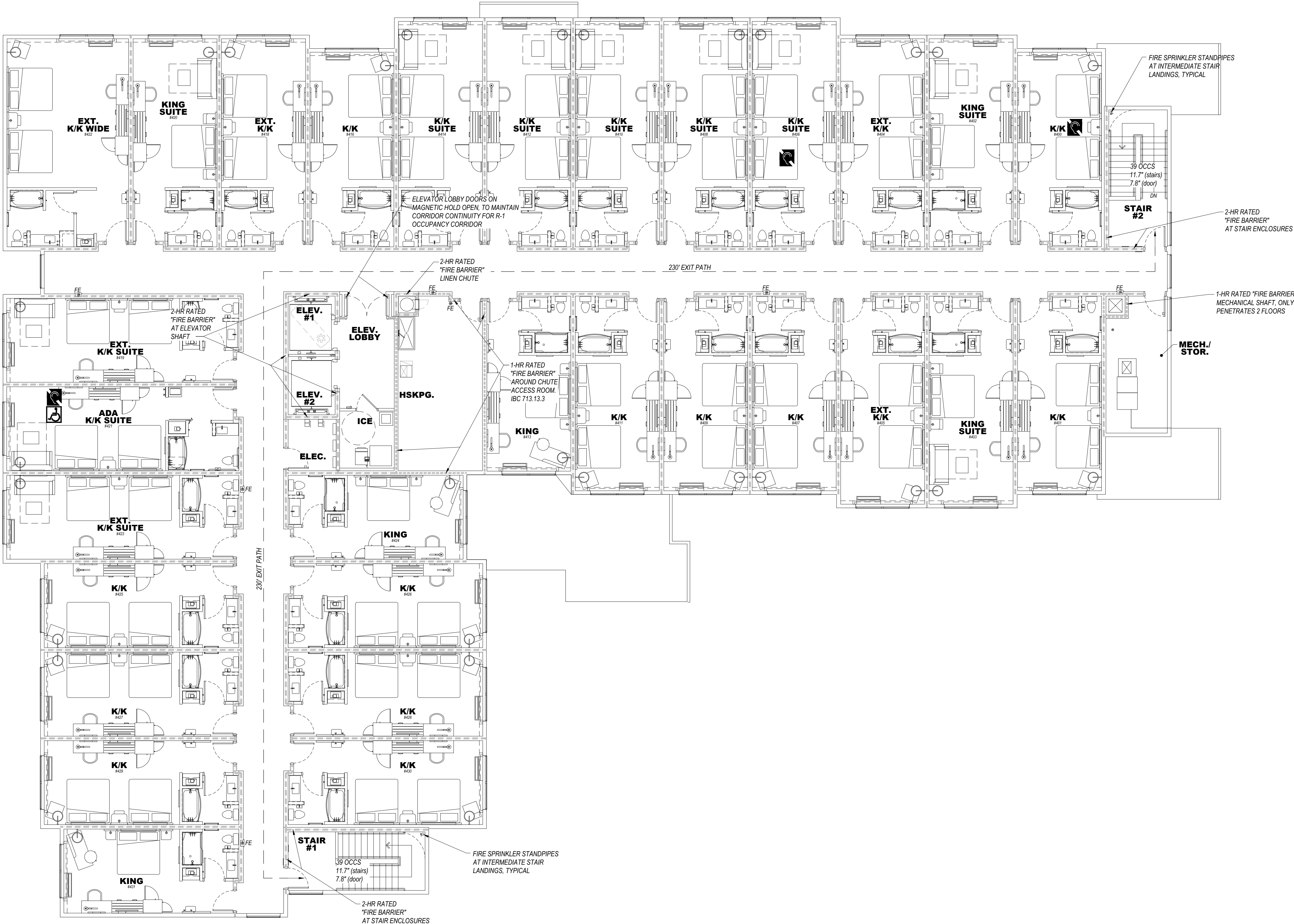
4TH FLOOR PLAN SCALE: 1/8"=1'-0" R-1 OCCUPANCY ENTIRE FLOOR
