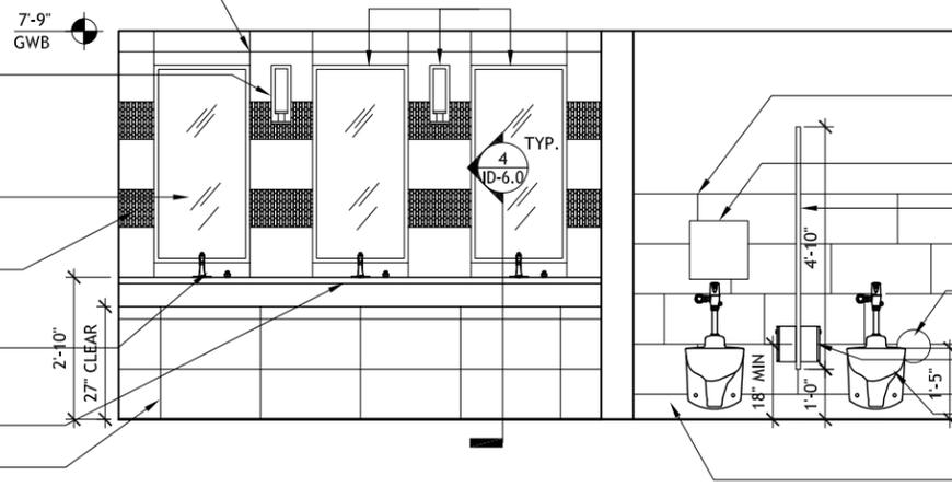
WAINSCOT HIGH TILE AS SPECIFIED; TILE TO BE OFFSET 1/3 LENGTH OF TILE, LAYOUT AS SHOWN. WALL ABOVE TO RECEIVE FINISH AS SPECIFIED. TOP EDGE OF TILE TO BE FINISHED WITH SCHLUTER JOLLY IN ANNOIDIZED ALUMINUM, TYP
