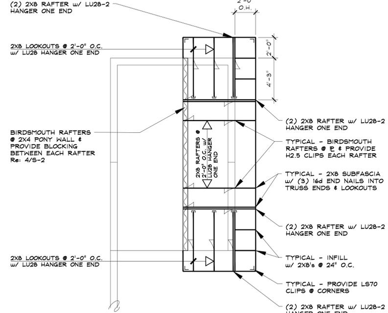
**2 LOWER ROOF FRAMING PLAN**
