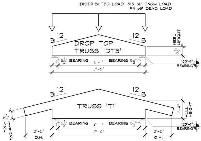
**8 MANUFACTURED TRUSS SCHEMATICS**
