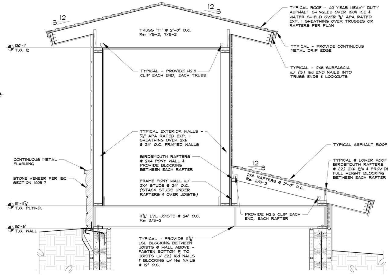
**4 BUILDING SECTION w/ DIAPHRAGM NAILING**
