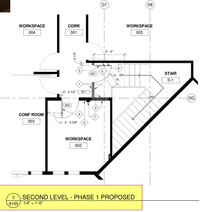
**DEMOLITION NOTES** A REMOVE PORTION OF EXISTING WALL FOR NEW DOOR. PATCH ADJACENT WALLS, CEILINGS AND
