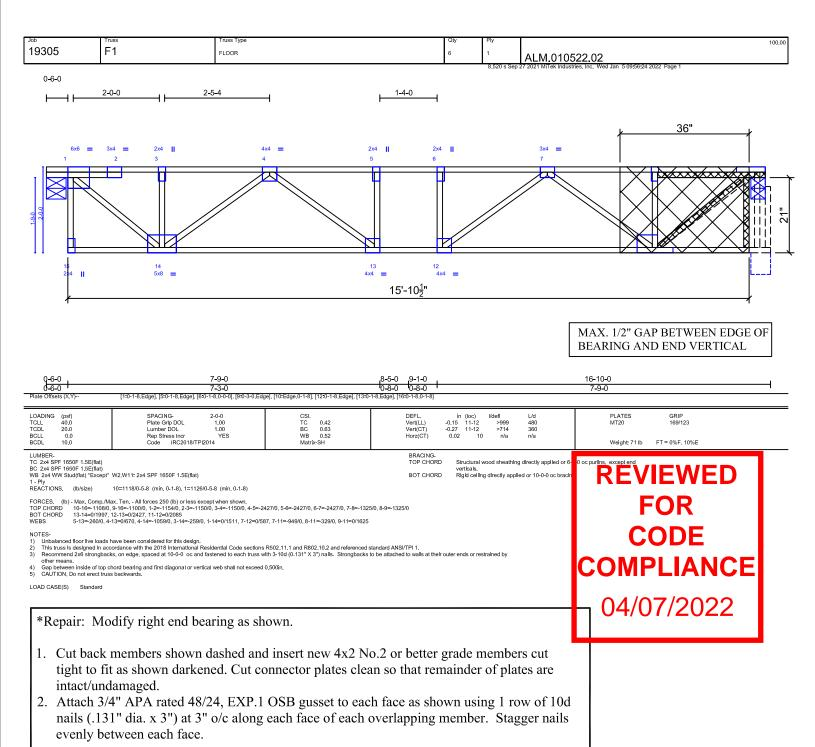
\* Engineering applies to repair only; refer to original sealed truss drawing for all other necessary truss documentation.
