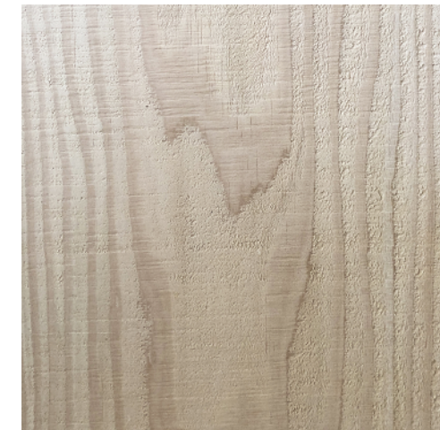
②.2 Roughsawn Solid DF - C Clear or better - Balcony Support and 2x6 Studs at Sauna Screen
