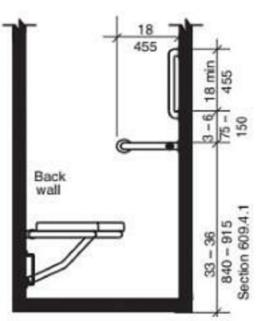
FIGURE 608.3.1(A) GRAB BARS IN TRANSFER-TYPE SHOWER - ELEVATION
