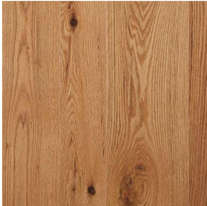
6.8 Red Oak Plywood -Millwork/ Interior Doors, Finish TBC.
